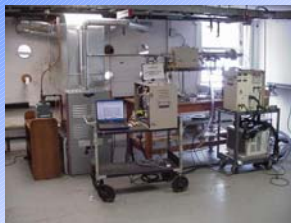
Utility Gas Fired Warm Air Furnace 81% AFUE NO x : 75ppm, SO 2 : ND, CO: 10ppm @ 3% O 2 Equiv.
