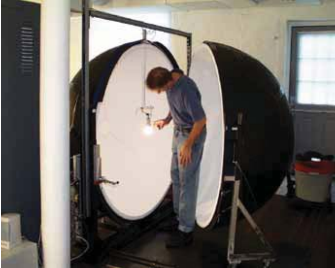
The Lighting Research Center's Laboratory Manager, Martin Overington, uses an integrating sphere to measure the overall light output of a light source.
