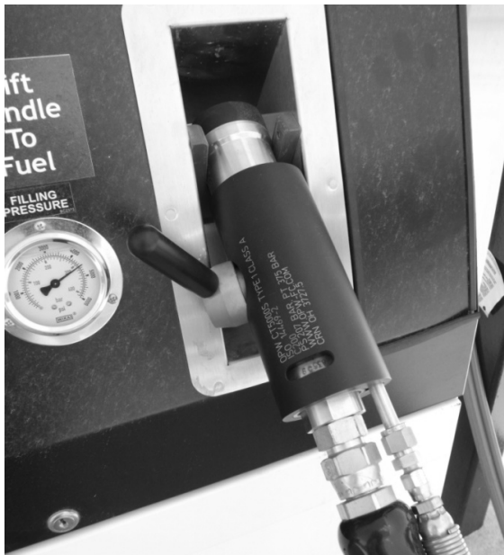
Figure 7. P36 CT5000 Type-1 compressed natural gas ball valve nozzle
