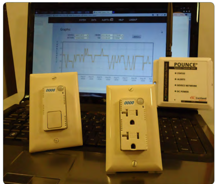
Showcased here is the POUNCE® system, developed by Cortland Research. The system includes a control unit, which is a web server and database that integrates and communicates with POUNCE® switches and outlets.
