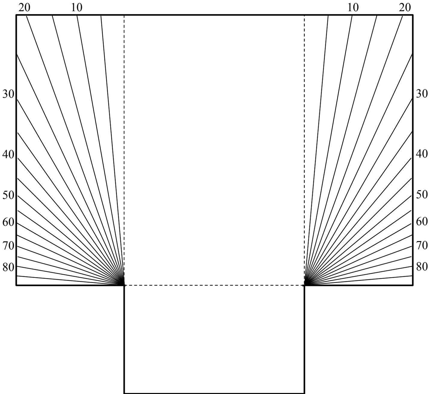
Figure 1: Template for building mounting props for solar panels
