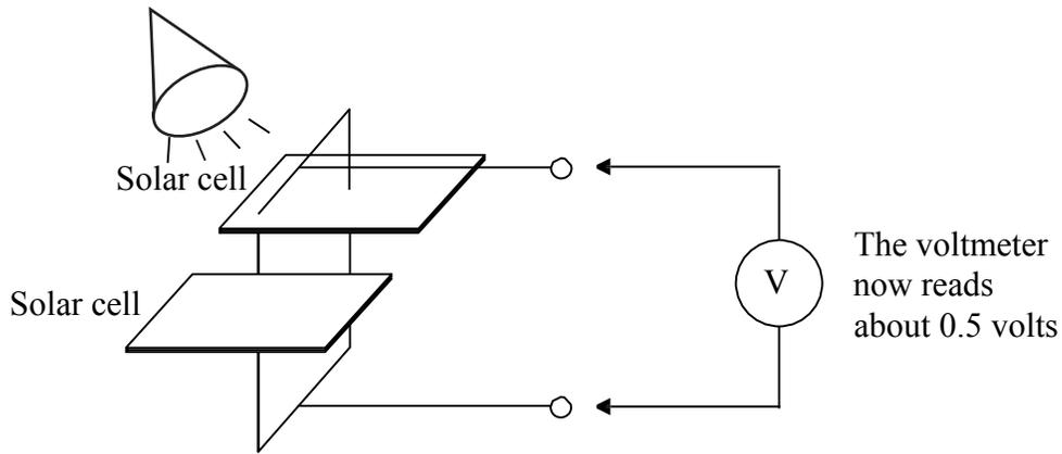
**Fact 3:** Two solar cells connected side by side (also known as “in parallel”) do not add their voltages together. They produce about 0.5 volts while under a bright light.
