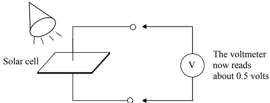
**Fact 1:** A single solar cell produces about 0.5 volts when placed under a bright light.
