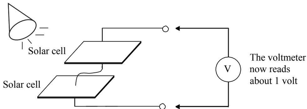
**Fact 2:** Two solar cells connected front to back (also known as “in series”) add voltages together to produce about 1 volt while under a bright light.
