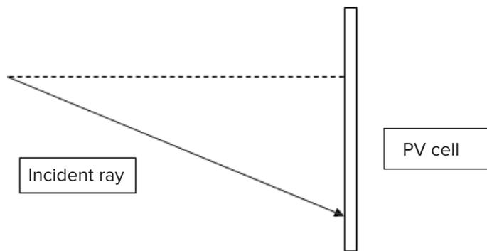
The horizontal line equals the length of the incident ray times the sine of the angle between the incident ray and the photovoltaic cell. It is the component of the incident ray that is perpendicular to the photovoltaic cell.
