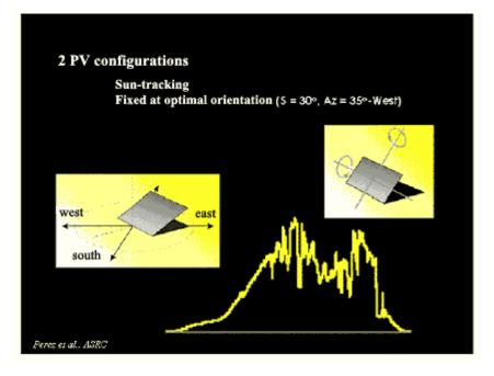
The graph at the bottom of the diagram shows typical solar energy collection by an ideal sun- tracking PV array from sunrise to sunset on a July day.
