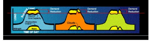
solar conditions are not good, backup energy supplies would be needed at that time (see middle graph), or alternatively, a reduction in consumer consumption would be necessary to guarantee that all resources above the red line are provided (see right graph).
