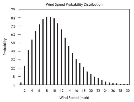
This curve shows the percentage of time that the wind blows at a given wind speed. The sum of the bars equals 100%. The taller the bar, the more likely it is that the wind will blow at the speed of that bar.
