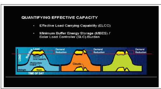
excess demand can be met by adding energy from the solar generation of electricity. When solar conditions are not good, backup energy supplies would be needed at that time (see middle graph), or alternatively, a reduction in consumer consumption would be necessary to guarantee that all resources above the red line are provided (see right graph).
