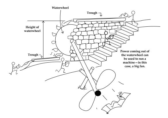
In this model, people climb stairs carrying buckets of water from the bottom trough of the waterwheel, and then they pour the water into the upper trough. The water flows down over the waterwheel, which has buckets attached to it that catch the water. The weight of the water in the waterwheel buckets makes the wheel spin. The power of the spinning wheel makes a machine such as the big fan spin.
