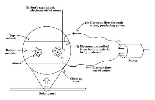
If wires from each layer are connected to a motor, the free electrons will flow from the top layer through the wire into the motor (making it spin) and then back through the wire connected to the bottom layer of the solar panel.
