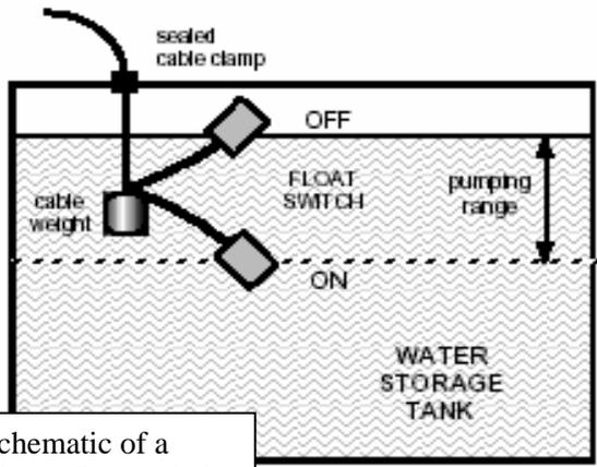
**Figure 11.** A schematic of a storage tank using a float switch.
