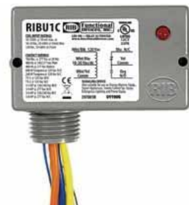
Figure 4-2 – Example of an external relay used when the load exceeds the amperage rating of the controller relay. The external relay must be rated higher than the load (image courtesy of Functional Devices, Inc.).
