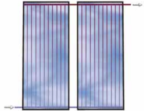
Figure 1-13 – Grid-style flat plate collectors plumbed in parallel (image courtesy of AET).
