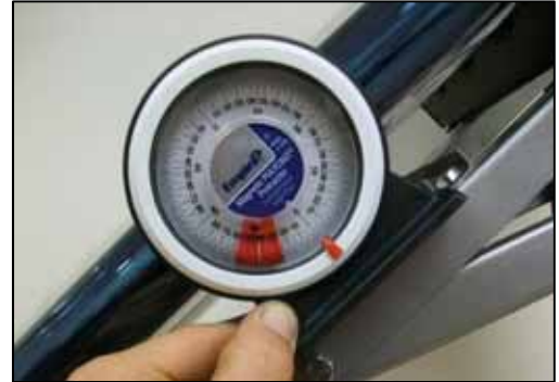
Figure 1-3 – An inclinometer is used to determine the tilt angle of a collector.
