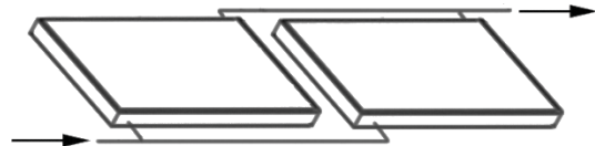
Figure 1-15 – Horizontal flat plate collectors plumbed in parallel
