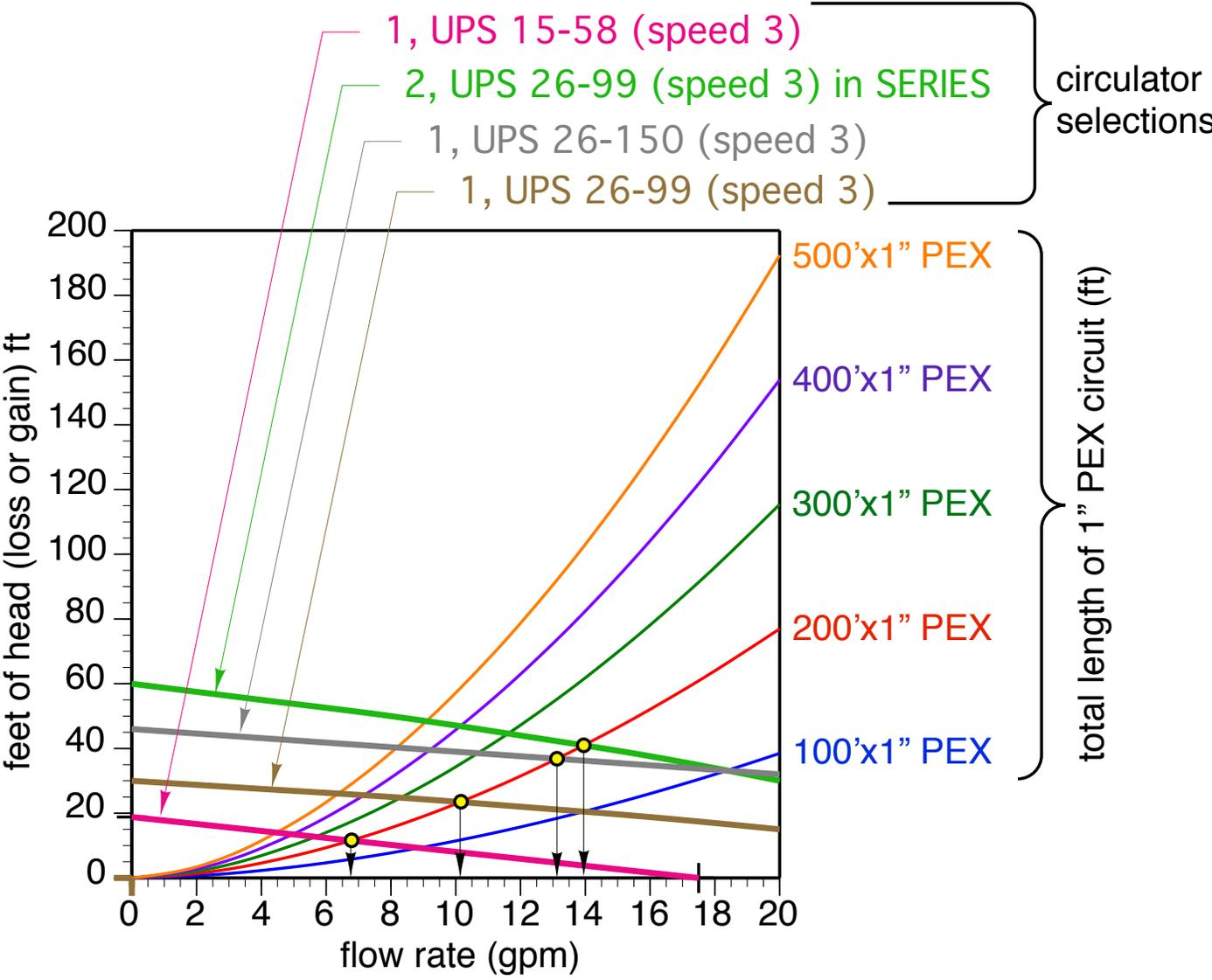
2 circulators in "close-coupled" series. **Double the head at each flow rate.**
