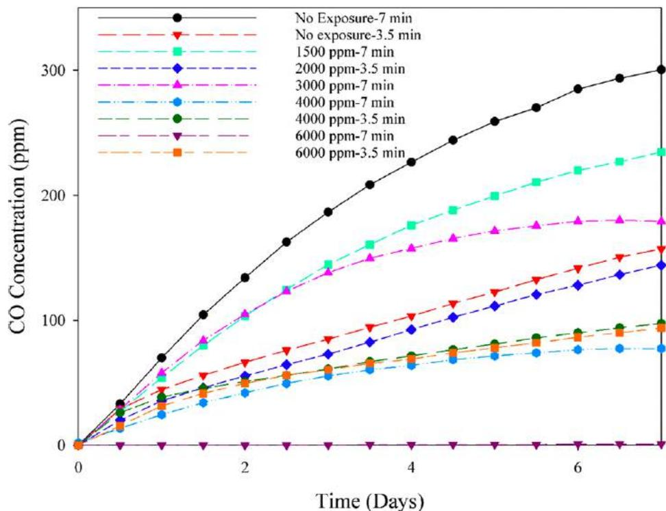
Figure 2. CO off-gas emission of wood fiber exposed at different ozone concentrations in a continuous process.
