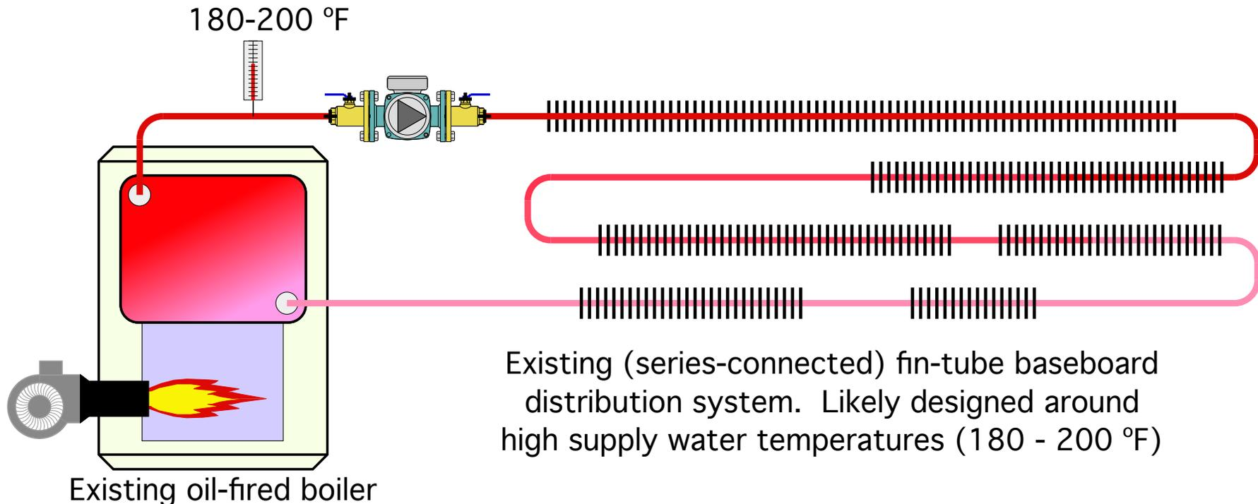
It's also likely that fin-tube baseboard will be connected in one or more series circuits as shown.
