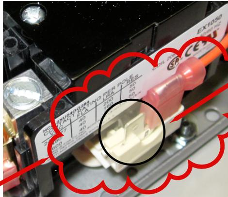
extra terminal on coil circuit of contactor
