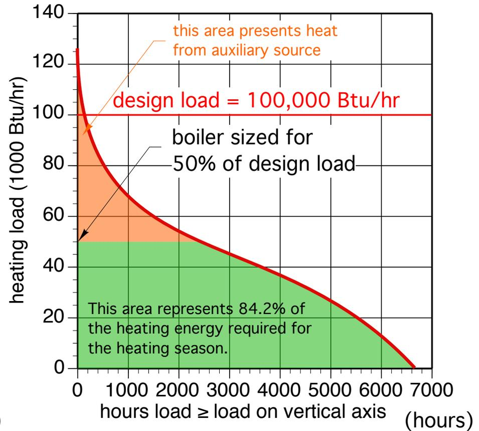
**Boiler sized @ 50% of design load provides about 84% of seasonal space heating energy.**
