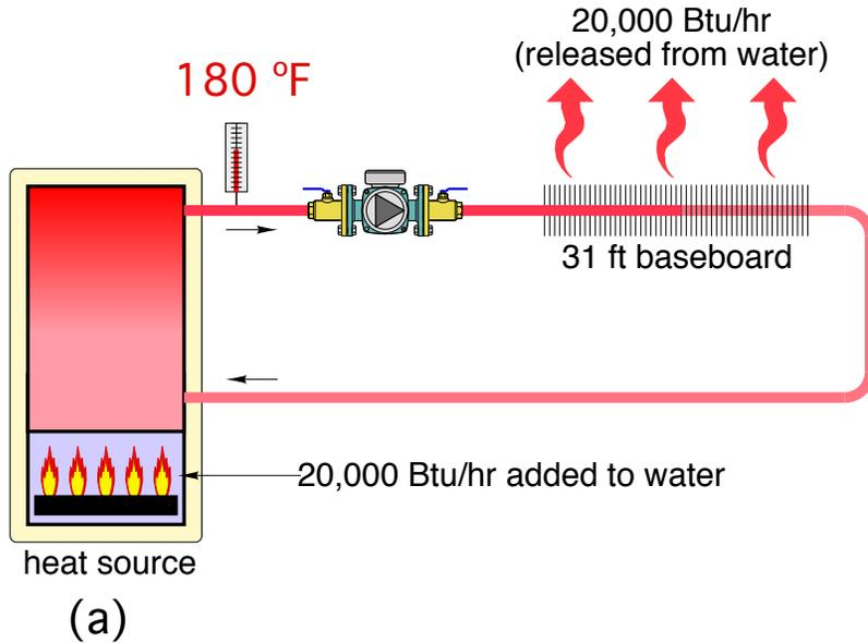
The greater the linear footage of baseboard, the lower the supply water temperature requirement.
