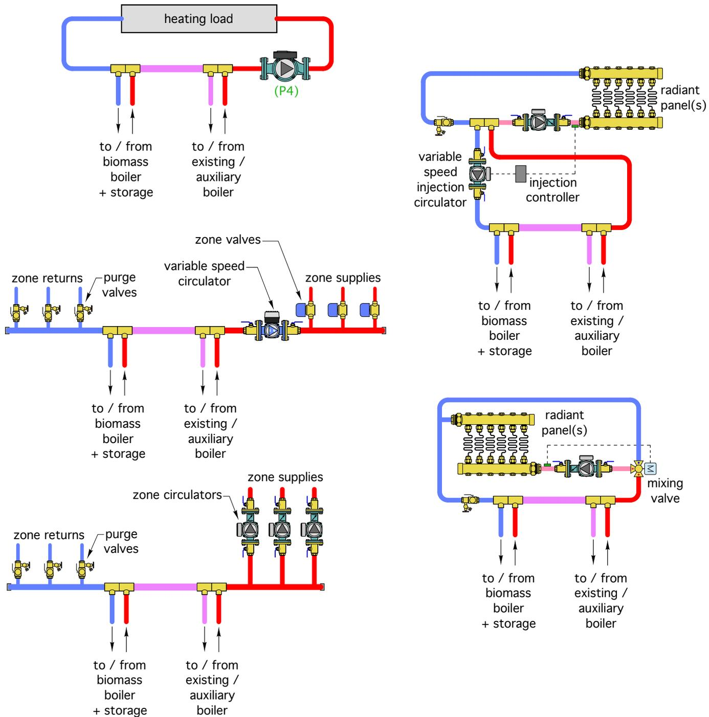
If distribution system can operate at low temperature remember to protect “conventional” boiler from sustained flue gas condensation
