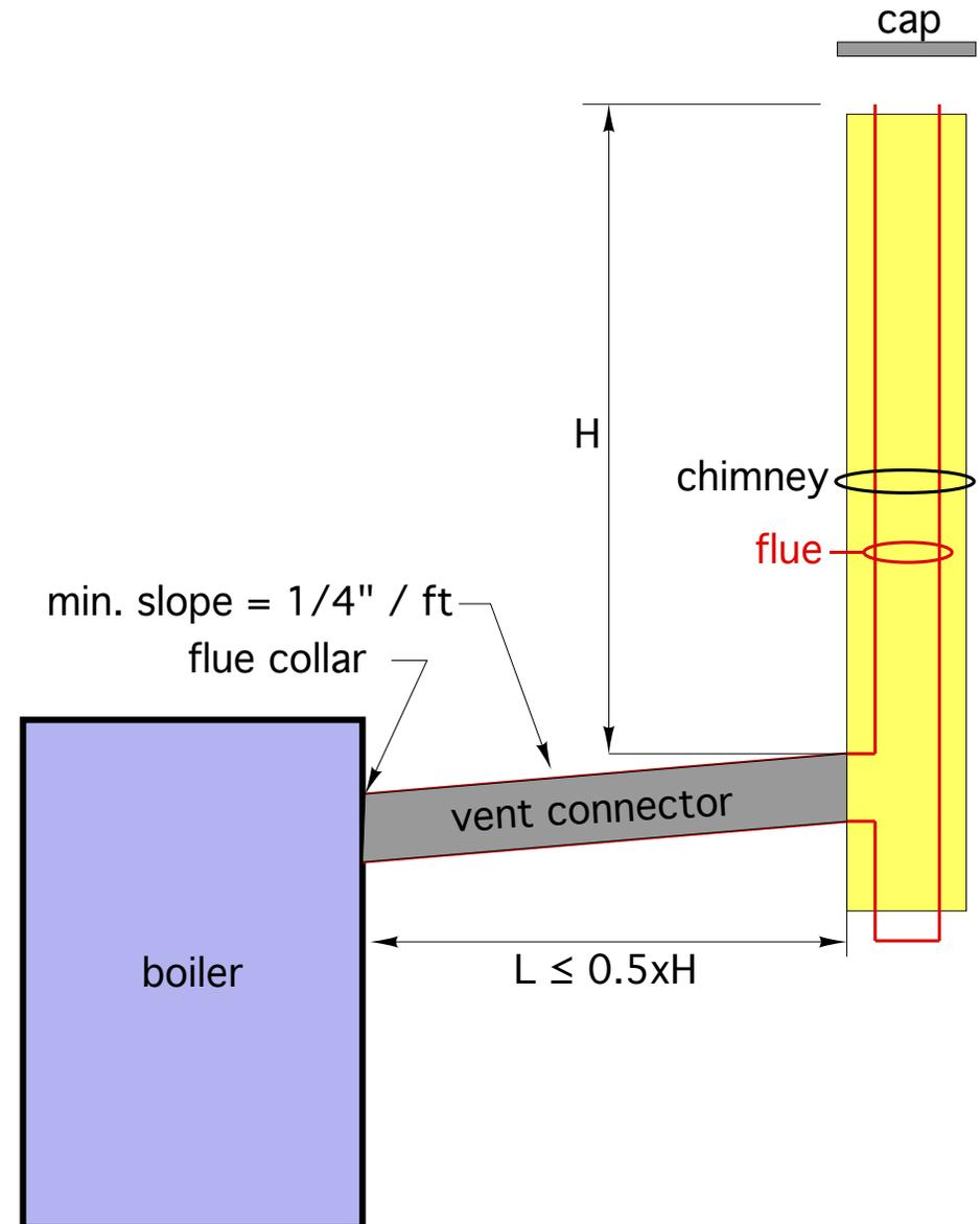
NYS code allows solid fuel appliances to be vented through 24 gauge (minimum thickness) galvanized steel piping.
