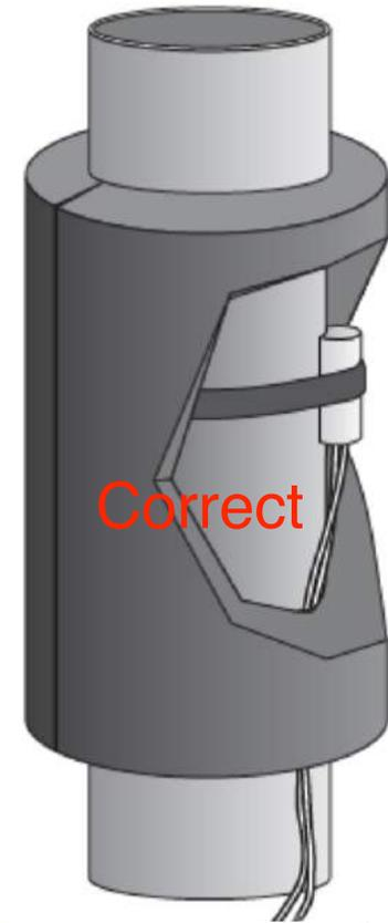
Some sensors have a concave shape to fit OD of pipe.
