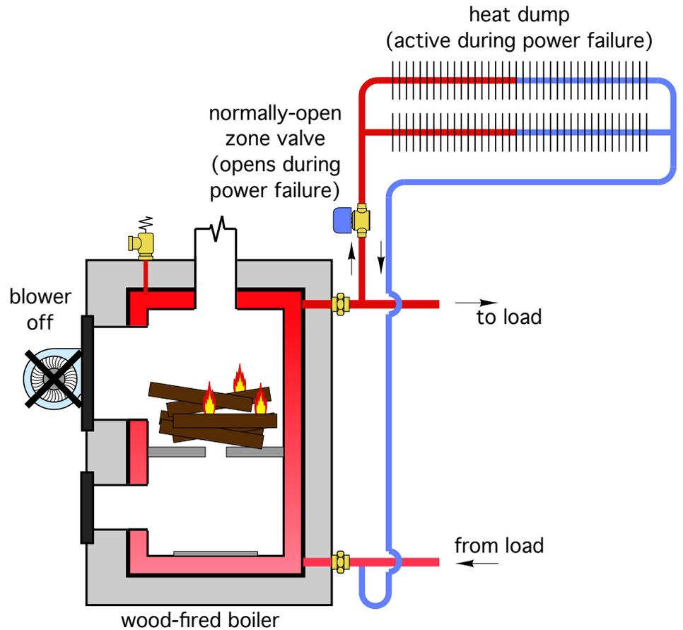
It's necessary to protect wood-fired boilers from low entering water temperatures.
