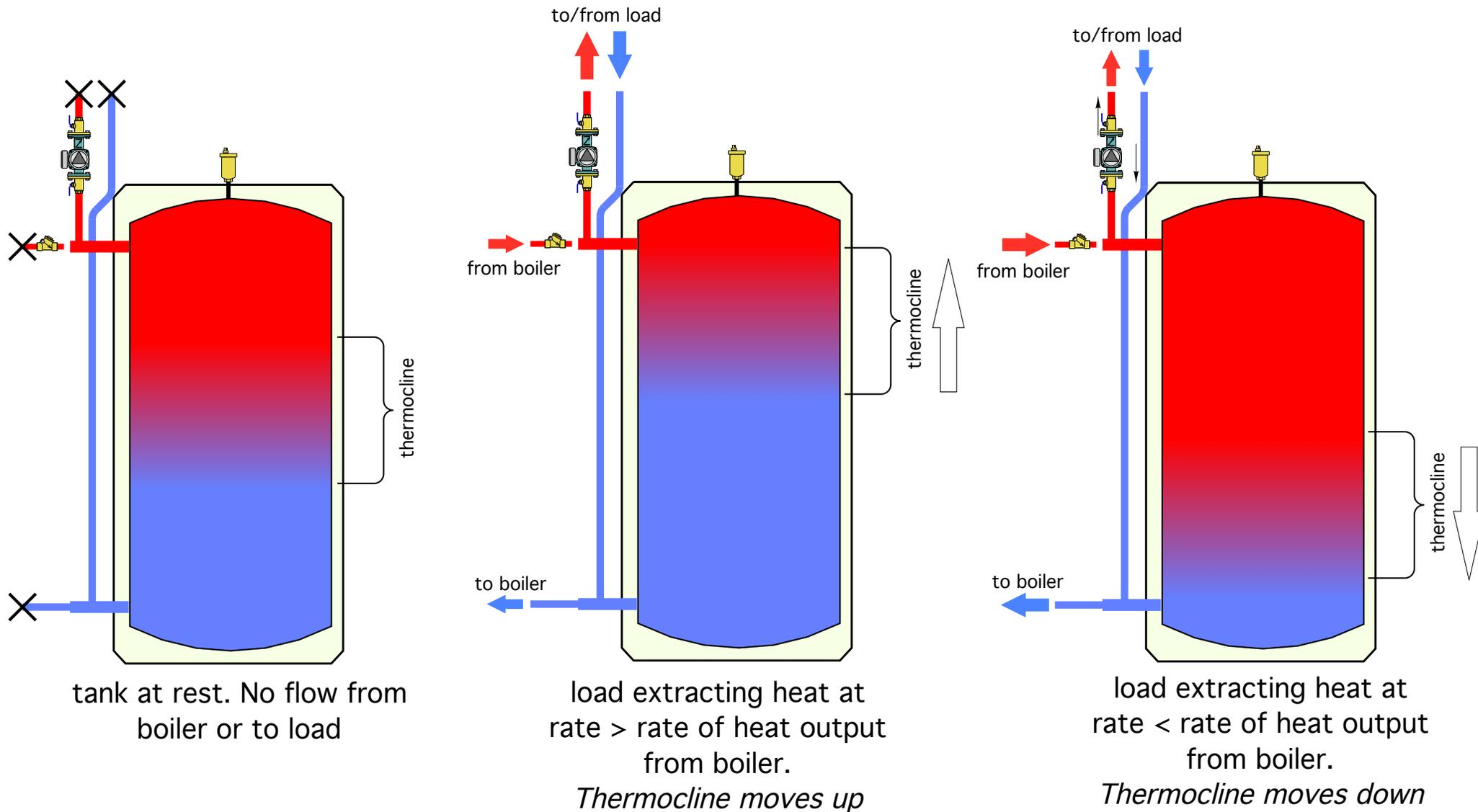
The pellet fired boiler should be turned on **before** the hot water is depleted from top of tank.
