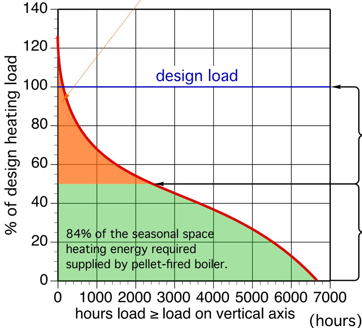
84% of the seasonal space heating energy required supplied by pellet-fired boiler.
