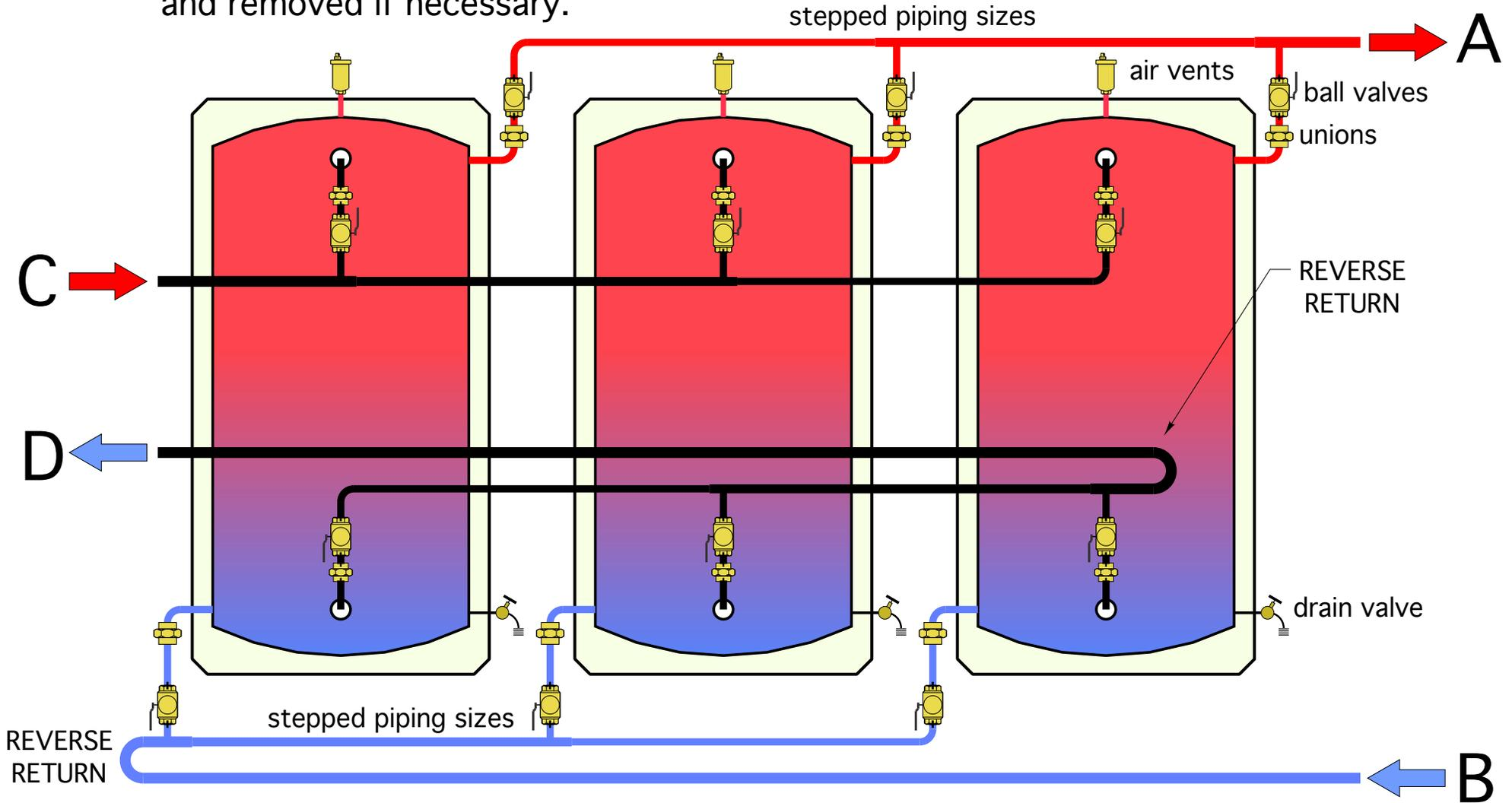
Could one of these tanks be removed - in tact- without disturbing the other tanks or piping?
