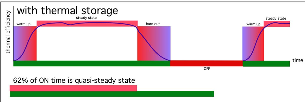
25 kW (85,300 btu/hr) rated pellet boiler supplying a heating load profile typical of an upstate NY house, with and without a 119 gallon thermal storage tank as part of the system.
