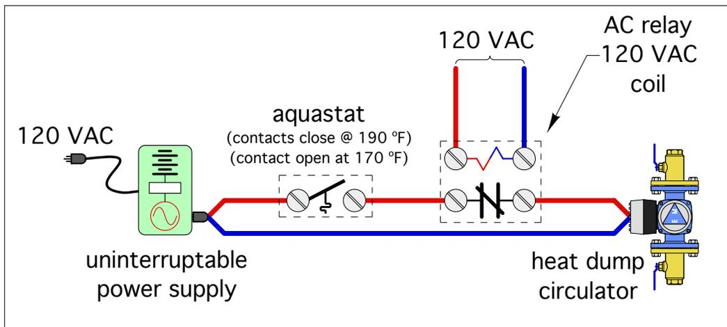
**The circulator allows possibility of heat dump being underneath the boiler.**
