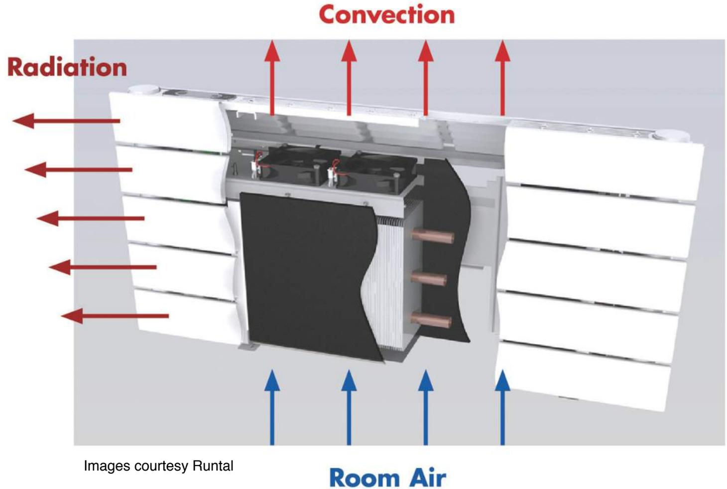
8 tube high x 31.5" wide produces 2095 Btu/hr at average water temperature of 104 °F in 68°F room
