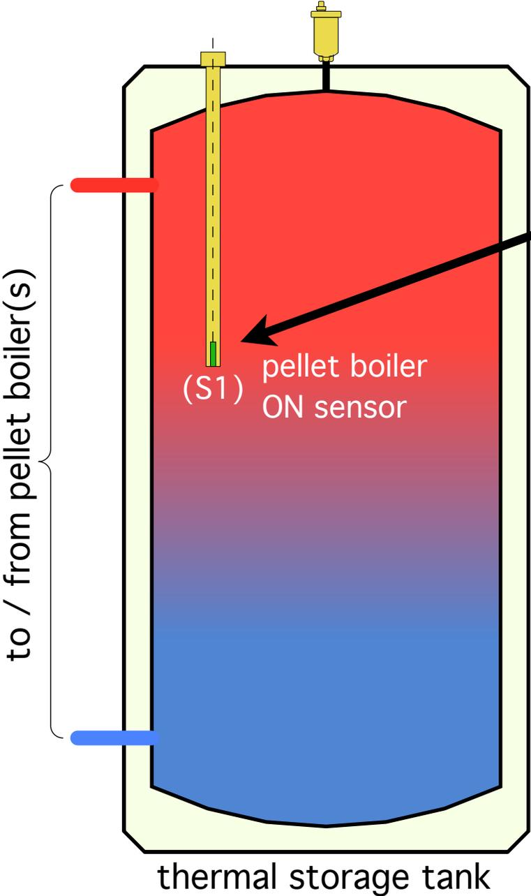
Sensor in vertical well detects “arrival” of rising cooler water. Turns on pellet fired boiler.
