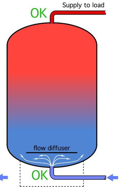
Flow diffuser installed
