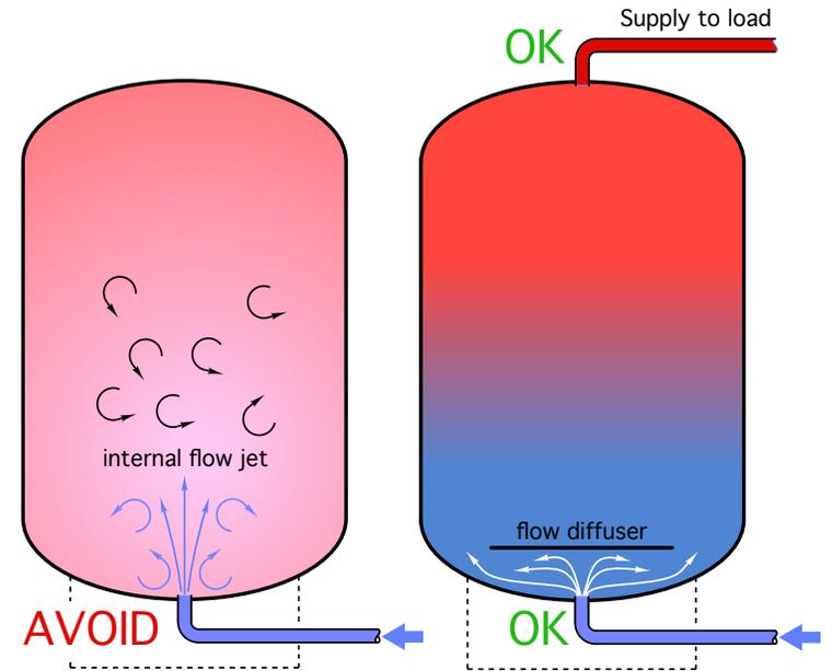
Do not route return flow into a vertical bottom connection (unless tank has inlet flow diffuser)
