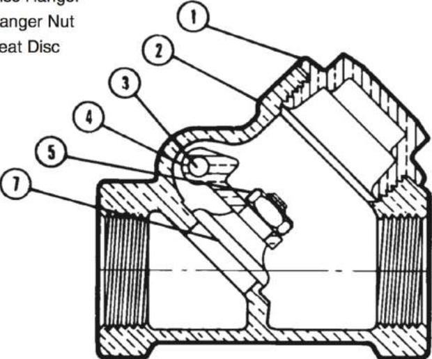
Only use a SWING CHECK valve here. Prevents reverse thermosiphon flow, but allows forward heat dump flow to tank in power outage.
