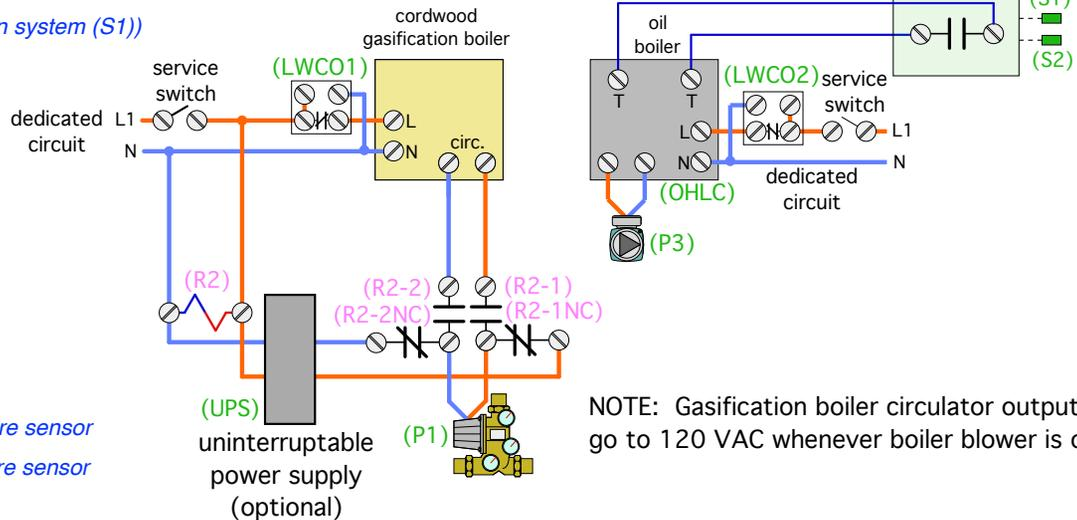
NOTE: Gasification boiler circulator output must go to 120 VAC whenever boiler blower is on
