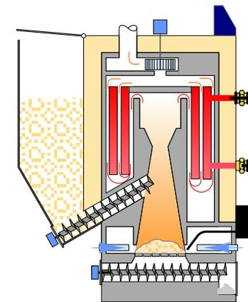
pellet boiler sized for 50% of design load
