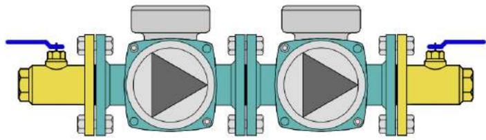
The pump curve for 2 circulators in series is found by doubling the head at each flow rate.
