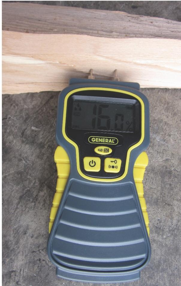
Proper assessment of the average moisture content of stacked cordwood should be based on measurements from several pieces taken from different areas of the stack. The end-grain moisture content along with the moisture content of internal fibers (wood samples are split open) should be measured. It's common for cordwood to have significantly higher internal compared to end-grain moisture content.
