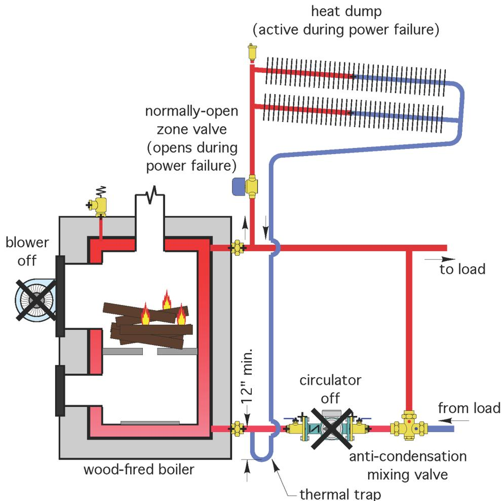
**Figure 2-7. Installed passive heat dump system**
