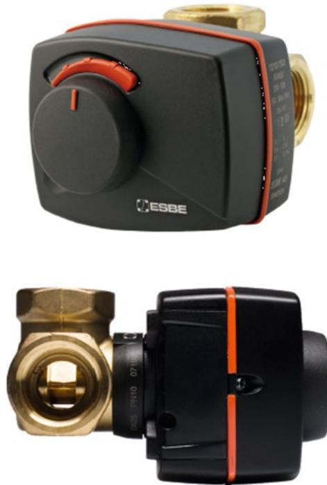
This assembly consists of a three-port, rotary mixing valve body coupled to an electrically-operated gear motor actuator. Three-way valve bodies, along with associated actuators are available in pipe sizes from three-quarter-inch to six-inch.
