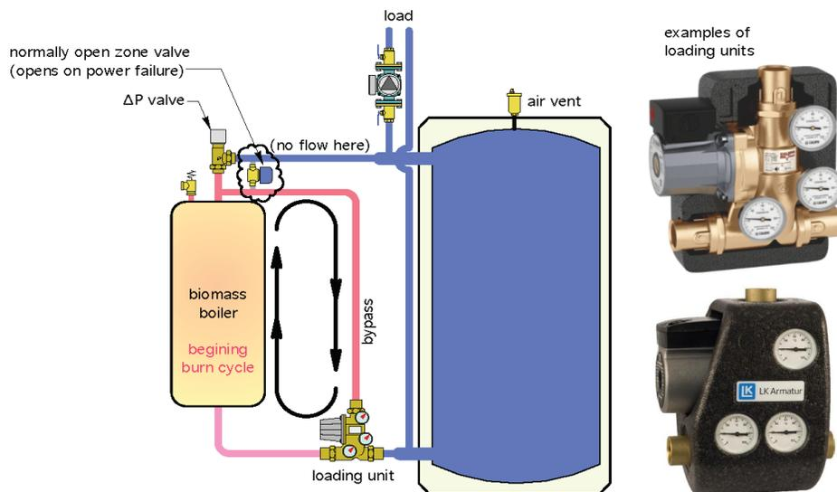
Loading units provide the same type of anti-condensation control as the previously described thermostatic mixing valve. They speed installation by combining the circulator and mixing valve into one assembly. They are also purchased with a specific actuating temperature setting. The actuating temperature can be changed by changing the thermostatic cartridge within the loading unit.
