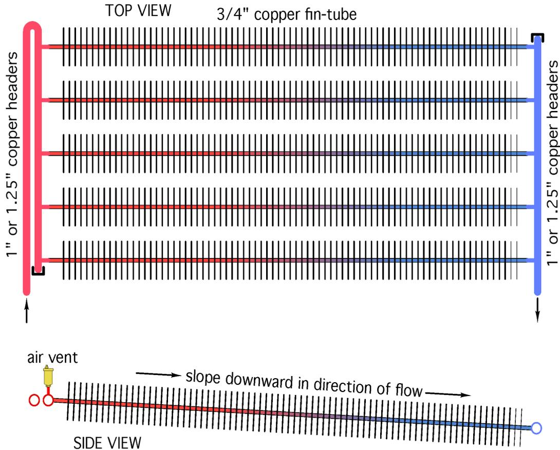
It's also possible to create an active heat dump in which flow is created by a small circulator powered by an uninterruptible power supply (UPS). The concept is shown in Figure 2-9.
