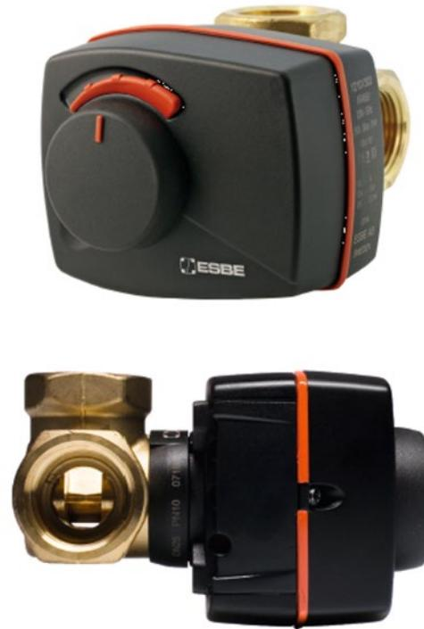
This assembly consists of a three-port, rotary mixing valve body coupled to an electrically-operated gear motor actuator. Three-way value bodies, along with associated actuators are available in pipe sizes from three-quarter-inch to six-inch.
