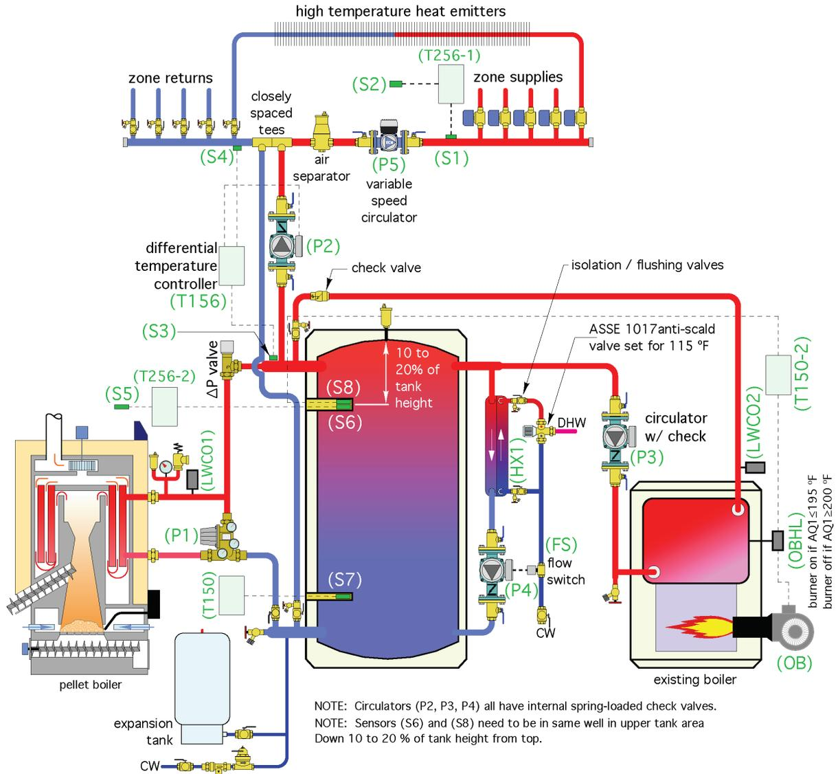
NOTE: Sensors (S6) and (S8) need to sense temperature at the same location in the tank and must be mounted in the same well, which should be located 10–20% of tank height down from top.
