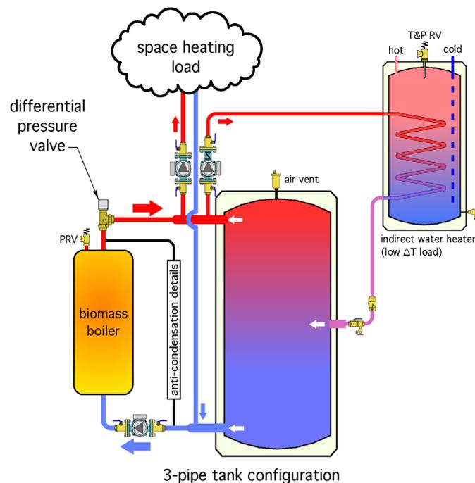
The three-pipe configuration supplies both space heating and indirect water heater loads from the upper tank header. The space heating return pipe connects to the lower tank header the same as with a two-pipe tank configuration. However, the return from the indirect water heater (representing a lower  $\Delta T$  load) connects to a mid-height tapping on the thermal storage tank.
