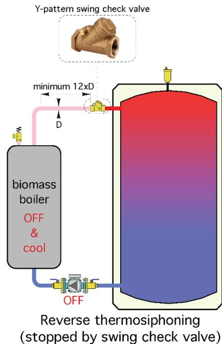
Swing check valves have minimal forward opening resistance. This is desirable because it allows them to pass forward thermosiphon flow, such as would develop if a power outage occurred and the boiler circulator was turned off while there was still wood burning in the boiler. This forward thermosiphoning is especially desirable in systems with cordwood gasification boilers due to the potentially high-residual fuel load in the combustion chamber when a power outage occurs.
