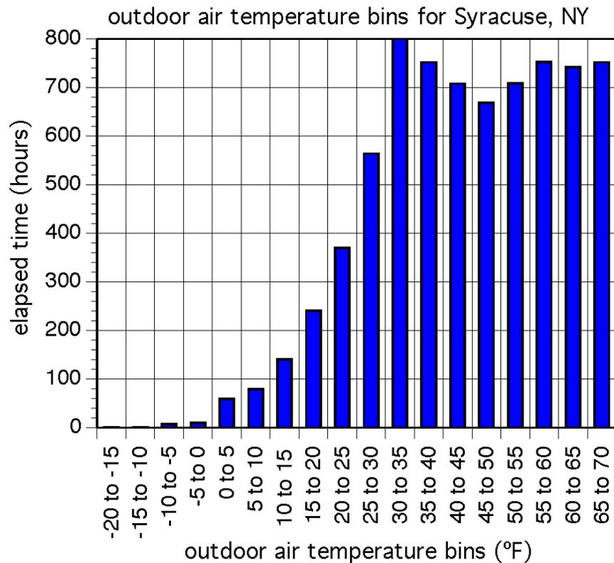
The 99 and 99.6% design dry-bulb temperatures for this location are 4.9 °F and -0.7 °F respectively. Notice that the vast majority of the hours in a typical year have corresponding outdoor temperatures well above these design temperatures. Under these conditions the heating load will be substantially lower than during the very infrequent design-load conditions.
