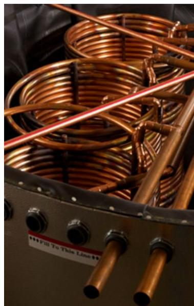
The thermal performance of coil heat exchangers is dependent on many variables including coil material, pipe diameter, coil height, diameter, flow rate, properties of the fluid flowing through the coil, and temperature stratification within the tank. Attempting to accurately calculate the theoretical heat transfer rates associated with natural convection can be very complex. For this reason, it is best to obtain heat transfer rate performance directly from the tank manufacturer.
