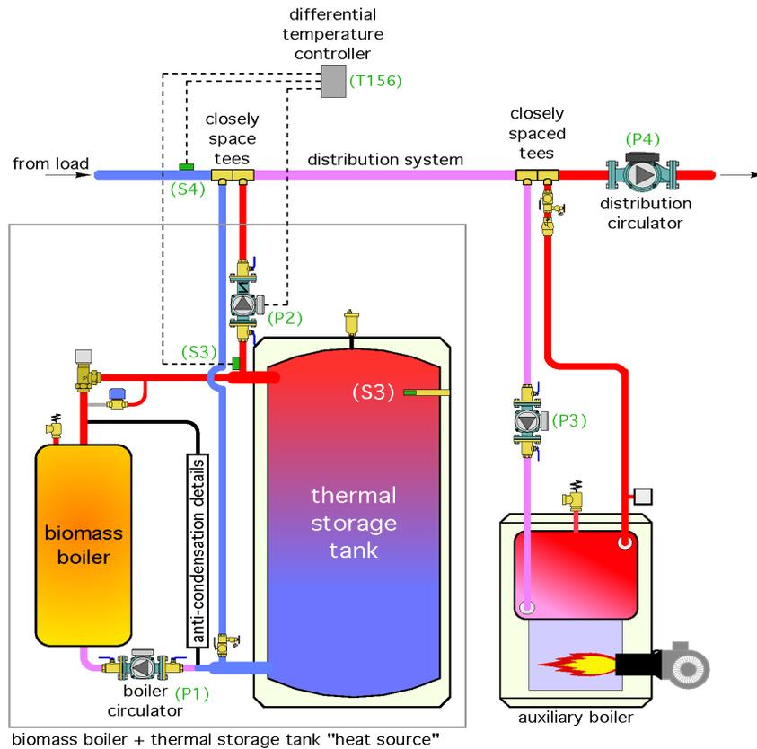
Sensor S3 measures the temperature at the upper tank header very close to the tank. This location allows S3 to perceive the presence of hot water from either the biomass boiler, if it's operating, or the upper portion of the tank, if the biomass boiler is off. Sensor S4 measures the temperature of water returning from the distribution system.
