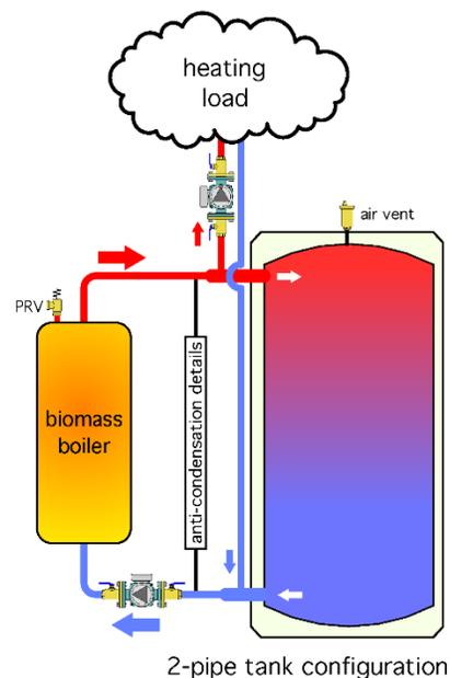
The two-pipe tank configuration holds two significant advantages relative to a four-pipe tank configuration.
