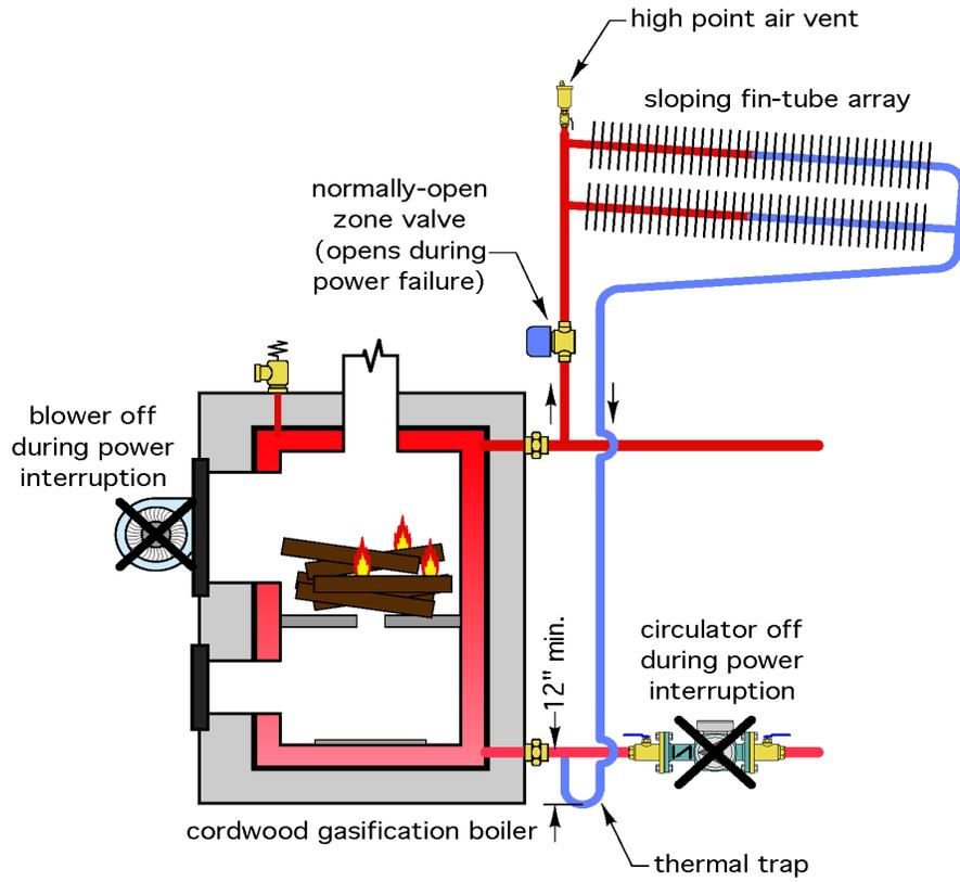
Figure 7-11. Finned-tube array above a cordwood gasification boiler as part of a passive heat dump
