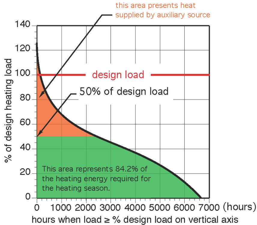
The green shaded area shows that 84.2% of the total seasonal heating energy use occurs when the heating load is 50% or less of design load. The remaining 15.8% of seasonal energy use occurs when the heating load is greater than 50% of design load. This implies that a boiler sized to 50% of design load could supply about 84% of the total seasonal heating energy requirement.
