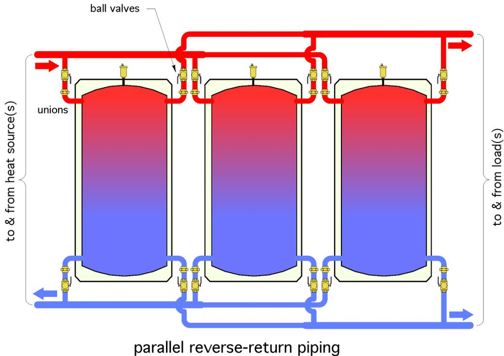
Reverse-return piping creates *approximately* equal flow rates through the tanks. If the designer wants assurance of exactly equal flow rates, two balancing valves should be substituted for two ball valves at each tank, one in the boiler circuit and the other in the load circuit. Balancing valves are typically more expensive than ball valves. The pipe sizes used for the headers connecting the tanks should be “stepped” to give approximately equal head loss per unit of length.
