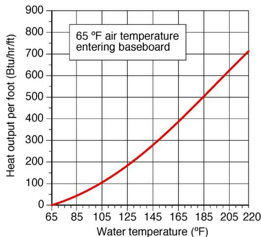
The average water temperature referenced in figure 6-2 is the average between the supply and return water temperature. The temperature drop across a baseboard circuit can vary widely depending on how the baseboard is piped. When several baseboards are piped in series, the temperature drop across the entire series circuit is typically in the range of 15–20°F.
