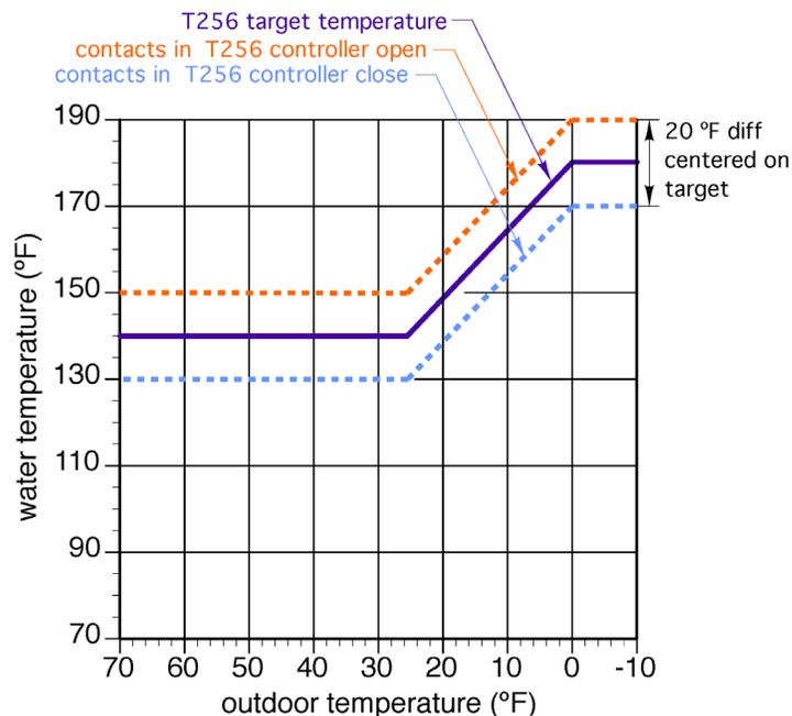
The minimum target water temperature has been limited to 140°F to prevent the oil-fired boiler from operating with sustained flue-gas condensation. If the oil-fire boiler was equipped with an anti-condensation mixing valve, the minimum water temperature could be lowered to 90°F.
