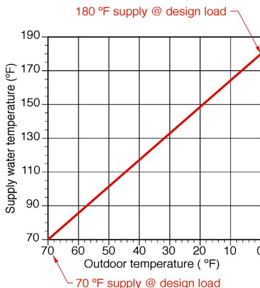
Outdoor reset can be very useful in extending the temperature cycling range of thermal storage tanks used in biomass boiler systems under partial-load conditions. Figure 6-21 shows an example.
