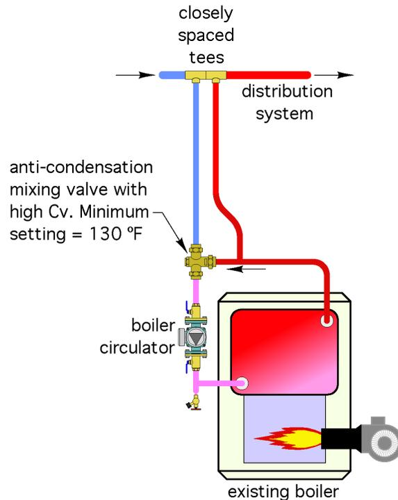
The anti-condensation mixing valve allows the existing/auxiliary boiler to operate at temperatures above the dewpoint of its flue gases, while still adding heat to the low-temperature distribution system. If the existing/auxiliary boiler is a modulating/condensing (mod/con) boiler, it is not necessary or desirable to use an anti-condensation mixing valve.
