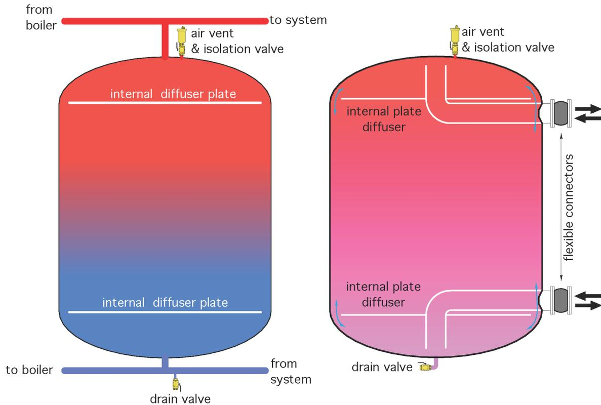
When the piping enters the side of the tank, it continues to an internal elbow that goes through the center of the plate diffuser. The flow impinges against the top of the elliptical end bell and spreads out symmetrically along its inner surface, eventually passing through the annular gap formed by the plate diffuser.
