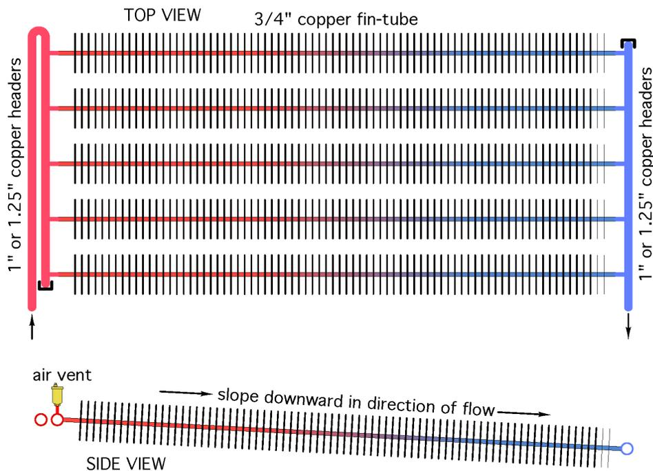
It's also possible to create a *powered* heat dump in which flow is created by a small circulator powered by an uninterruptible power supply. This is different from the use of a UPS to keep the boiler and boiler circulator operating as normal. The concept is shown in Figure 7-13.
