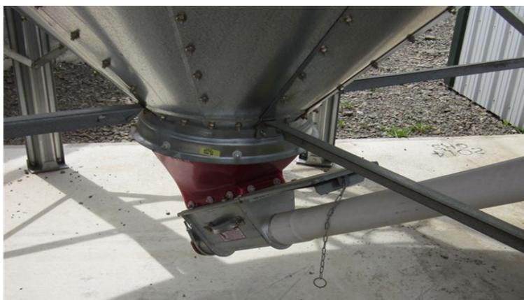
Regardless of the type of pellet transport system used, it is critically important that the pellet receiver assembly be designed, installed, and maintained so that precipitation cannot enter.
