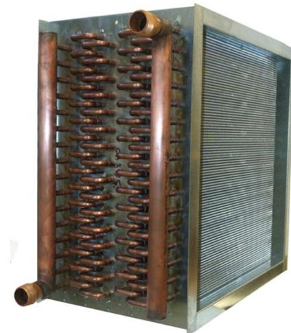
The coil must also be evaluated for its air-side static pressure drop in relationship to the furnace's blower and ducting system. The coil's air-side static pressure drop must be low enough that the existing furnace blower can provide adequate air flow to the building with that air flow passing through the new coil. Furnace specifications typically list the static pressure capability of the blower along with associated air flow rates.
