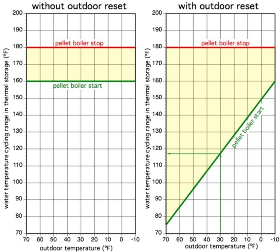
The graph on the left represents a situation in which the pellet boiler starts as a sensor in the thermal storage tank drops to 160°F and continues to operate until the temperature at the sensor reaches 180°F. Neither of these temperatures change as the outdoor temperature changes.
