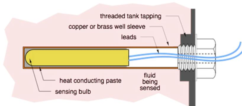
Thermal paste reduces thermal resistance between the inside of the well and the sensor, and temperature measurement accuracy improves. Thermal paste also reduces the time lag between changes in temperature of water surrounding the well and when those changes are detected by the sensor.
