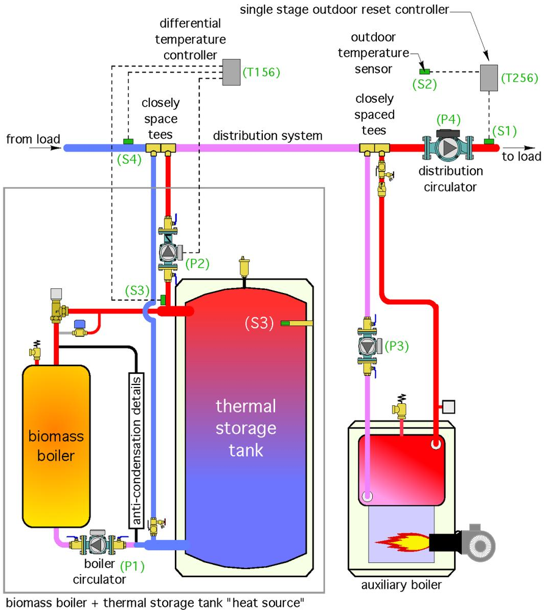
The combination of the differential temperature controller (T156) and outdoor reset controller (T256) addresses all three previous stated objectives for controlling heat input to the distribution system from both heat sources. Figure 7-25 shows how these devices can be combined electrically, along with circuitry that signals when a heating demand is present.
