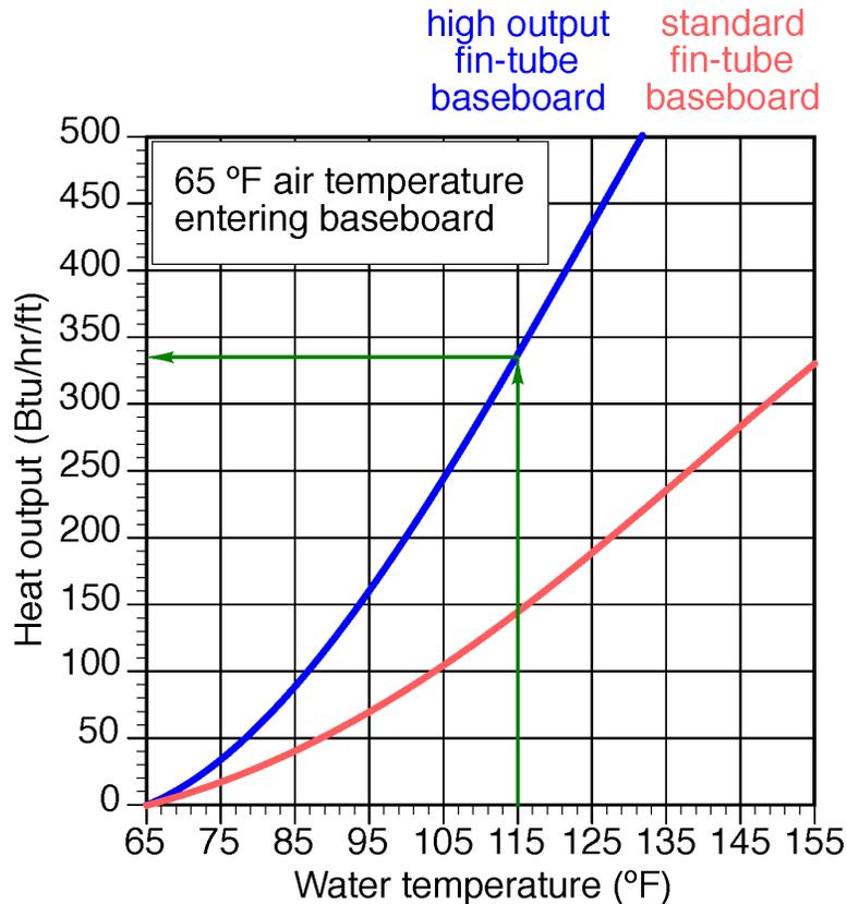
The steps of the previous procedure can be modified to determine the amount of high-output, finned-tube baseboard that is required to reduce the supply water temperature to the system under design load.
