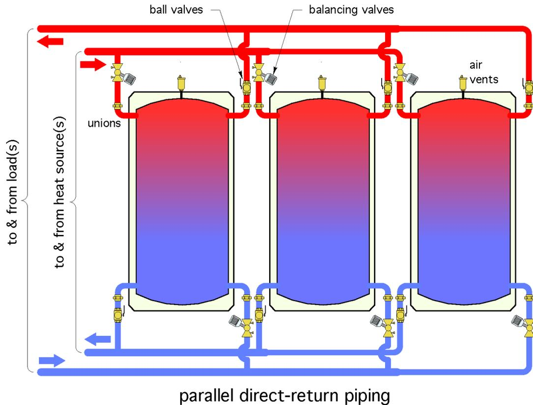
The pathways the fluid follows through each tank have different lengths. Through the left tank the pathway is the shortest, longer in the center tank, and longest through the right side for both the boiler circuit and load circuit.
