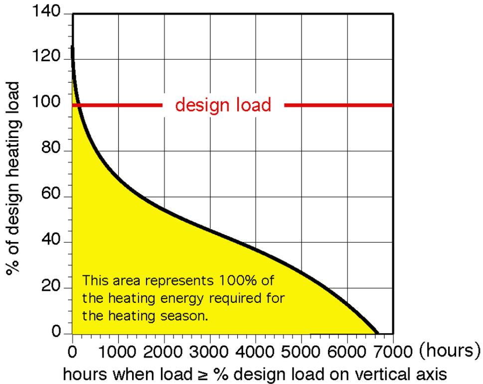
The vertical axis of this graph represents the percent of the design-heating load. The horizontal axis shows the hours during which the heating load is equal to or greater than the percent of design-heating load on the vertical axis. Although this graph is specific to the statistical weather data for Syracuse, NY, the characteristic curved shape of the shaded area is typical of other cool or cold climate locations.
