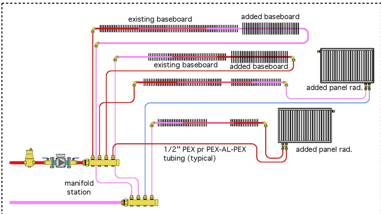
In this situation the existing series circuit was divided into four branch circuits. Supplemental heat emitters were added to each of these circuits. Two of the circuits received additional fin-tube baseboard, and the other two received panel radiators. These heat emitter selections are provided only to illustrate that multiple types of supplemental heat emitters can be used depending on available wall space, budget, and aesthetic preferences.
