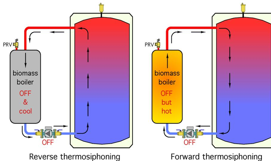
Reverse thermosiphoning can be stopped by installing a high-quality swing check valve in the piping near the upper tank connection. A "Y-pattern" swing check valve, as shown in Figure 7-4, is recommended over swing check valves with vertical discs. The latter have, at times, demonstrated an inability to block reverse thermosiphon flow due to a slight gap between the valve's internal disc and its seat.
