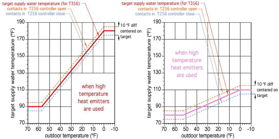
The following suggested initial controller settings assume low-temperature heat emitters that require a supply temperature of 110°F under design load conditions (0°F outdoor temperature).
