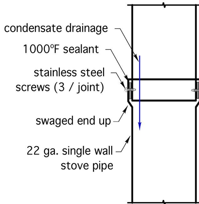
Most codes require single-wall vent connector piping to be at least 18 inches away from any combustible materials. NFPA standards allow clearance distance reductions when specific types of thermal shielding are used.
