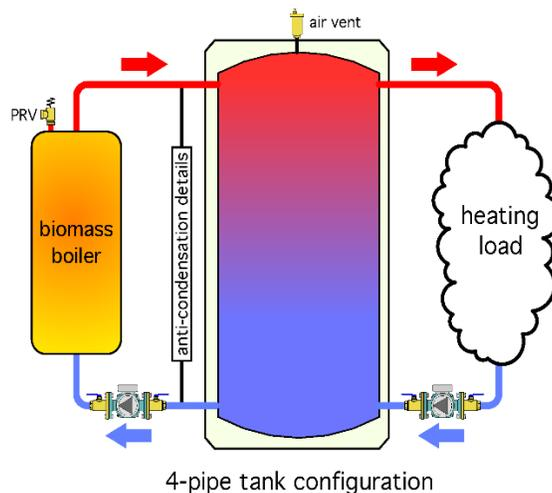
In a four-pipe tank configuration, all the energy flowing from the biomass boiler to the load must pass through the thermal storage tank. The hotter water entering the tank from the boiler tends to stay in the upper portion of the tank, although there will be some mixing which is counterproductive to good temperature stratification. The cooler water returning from the load tends to stay in the lower portion of the tank.
