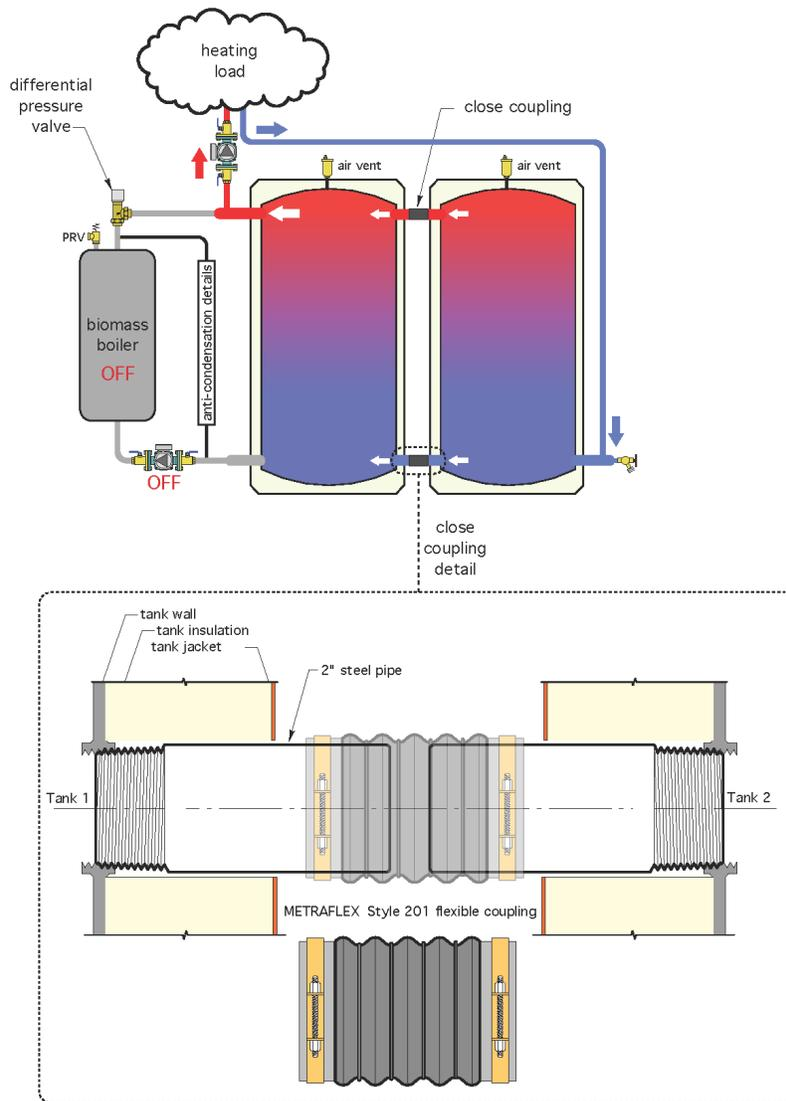
The coupled tanks shown in Figure 5-27 are a close approximation of the two-pipe configuration described earlier. The flow rate passing through the tanks will always be the difference between the boiler flow rate and the load flow rate. This tank configuration is significantly less expensive than previous discussed configurations but does not allow each tank to be isolated and serviced.
