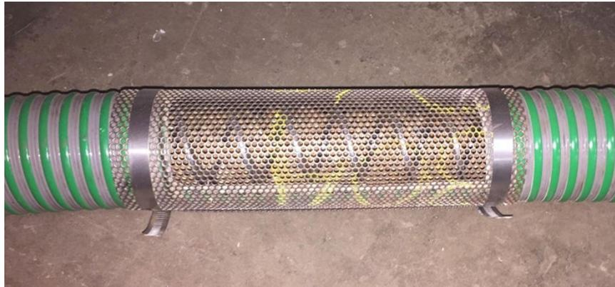
As the pellets pass the screen, fine particles caused by fractured pellets fall through the openings. This reduces fines within the boiler's stoker queue and stoker auger. If a fines screen is used it should be supported above a collection pail. The pail should also be covered to prevent dust emitted from the screen from becoming airborne within the mechanical room. The collection pail should be periodically checked for accumulation and emptied.
