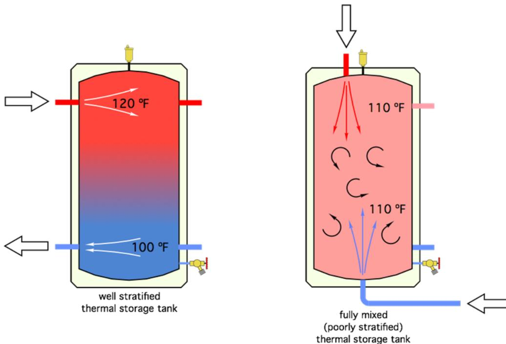
Assume that both tanks are identical in volume, shape, and insulation. The tank on the left exhibits good temperature stratification. The water temperature at the top is 120 °F, and the water temperature at the bottom is 100 °F. Assuming a symmetrical temperature profile from top to bottom, the average water temperature in the tank is 110 °F. The tank on the right has been subject to mixing such that the entire tank contains water at 110 °F.
