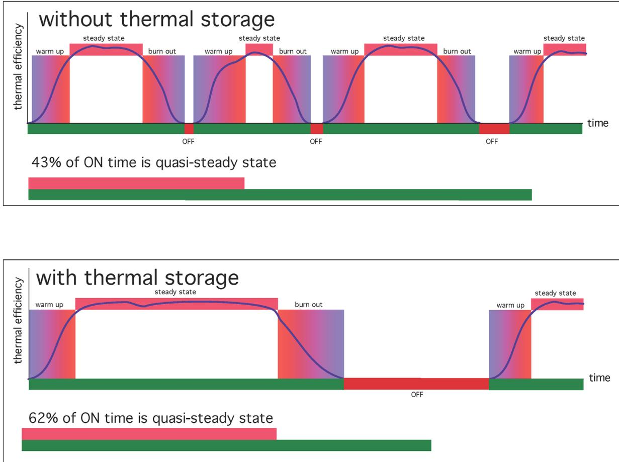
Figure 3-1 shows the percentage of elapsed time the boiler operates at or close to steady state combustions conditions. The scenario with longer and less frequent boiler cycling yields a higher percentage of quasi-steady state combustion. The higher this percentage, the higher the overall integrated efficiency of the boiler and the lower its emissions.
