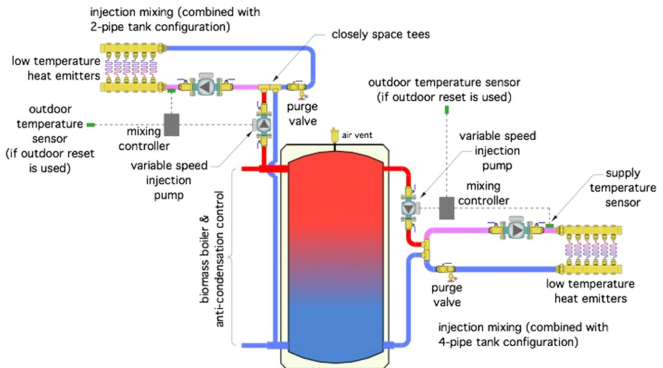
The variable speed pump can be a standard wet-rotor circulator with a permanent split capacitor (PSC) motor or a circulator with an electronically commutated motor (ECM).
