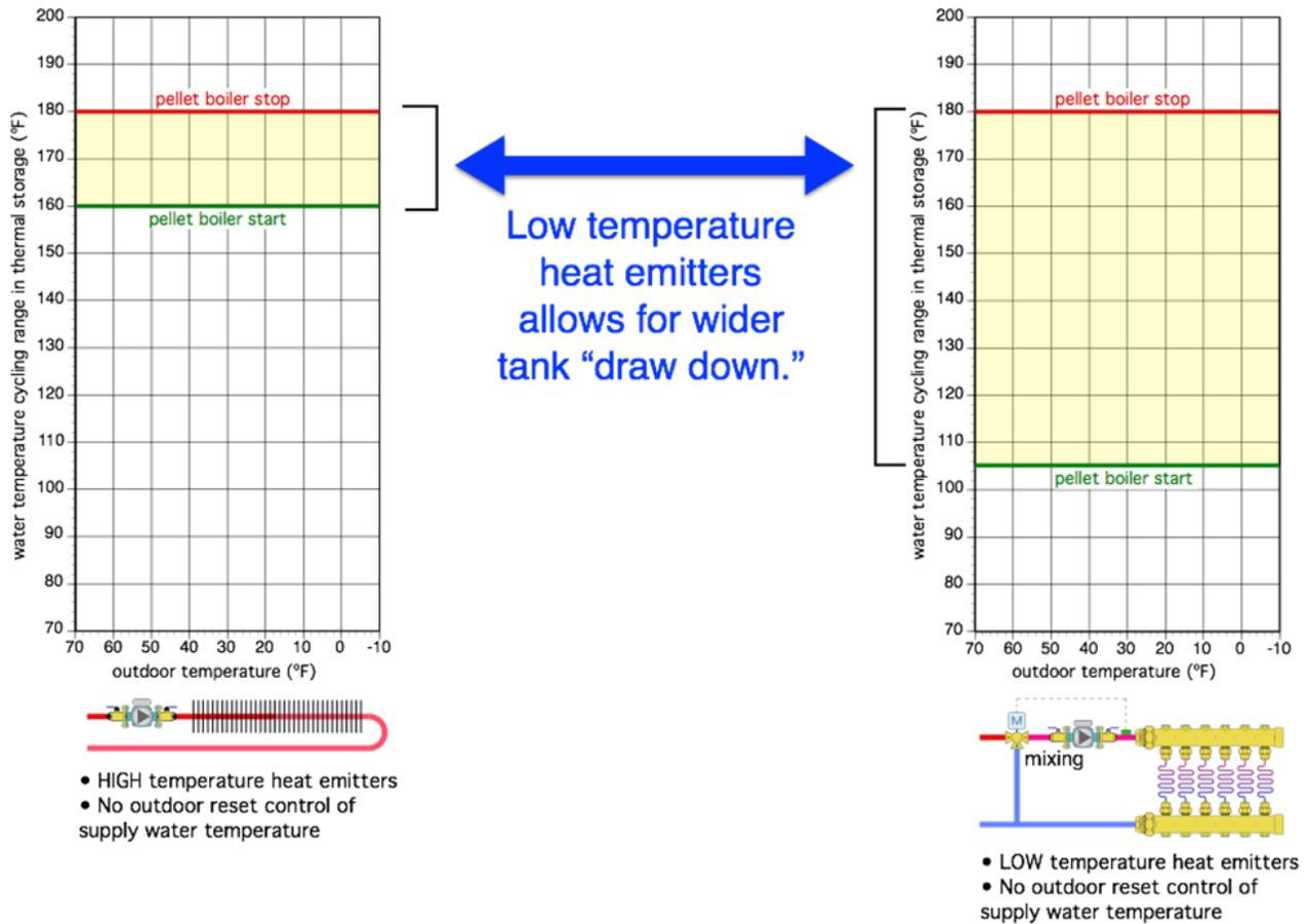
The graph on the left represents a system with fin-tube baseboard that has been sized to provide design-load heat output at a water temperature of 180 °F. In this case, the pellet boiler is turned on when the tank sensor temperature drops to 160 °F and remains on until the sensor temperature climbs to 180 °F. The shaded yellow area on the graph shows that this temperature cycling range is independent of outdoor temperature.
