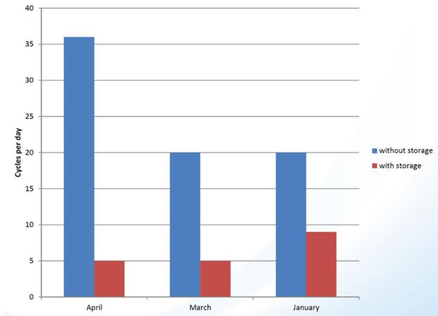
Notice the significant reduction in boiler cycles per day when storage is used, especially under the partial load conditions associated with April and March operation.
