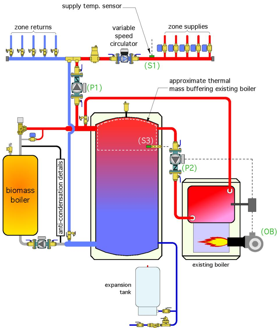
The existing boiler is piped across the upper portion of the thermal storage tank. This allows the upper portion of the tank to buffer the operation of the existing boiler. When the load is space heating, the existing boiler is not meant to continuously maintain the upper portion of the thermal storage tank at a minimum temperature.
