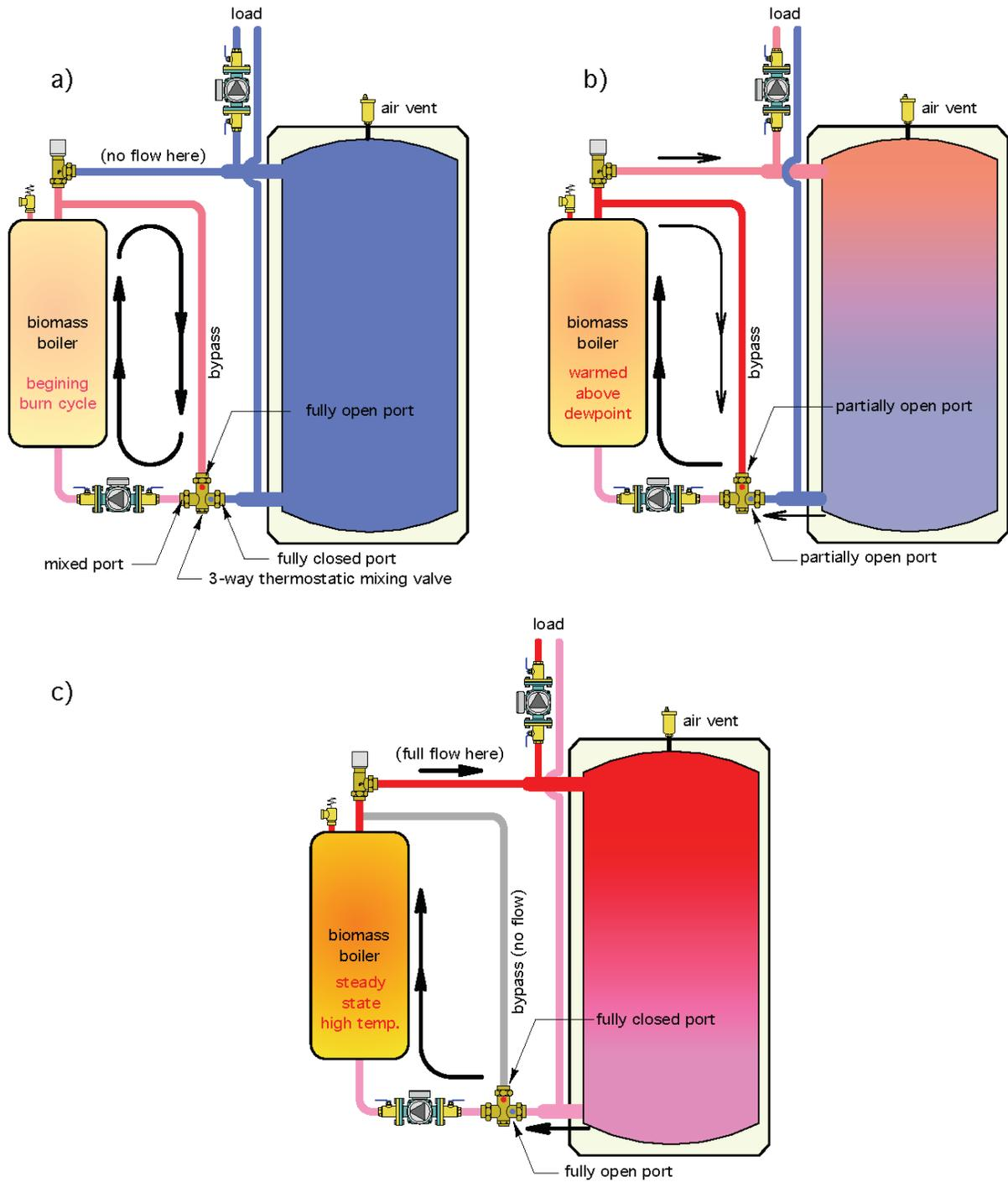
This process works in reverse as the boiler's heat production rate decreases. The objective remains the same—to keep the boiler's inlet temperature warm enough to prevent sustained flue-gas condensation.
