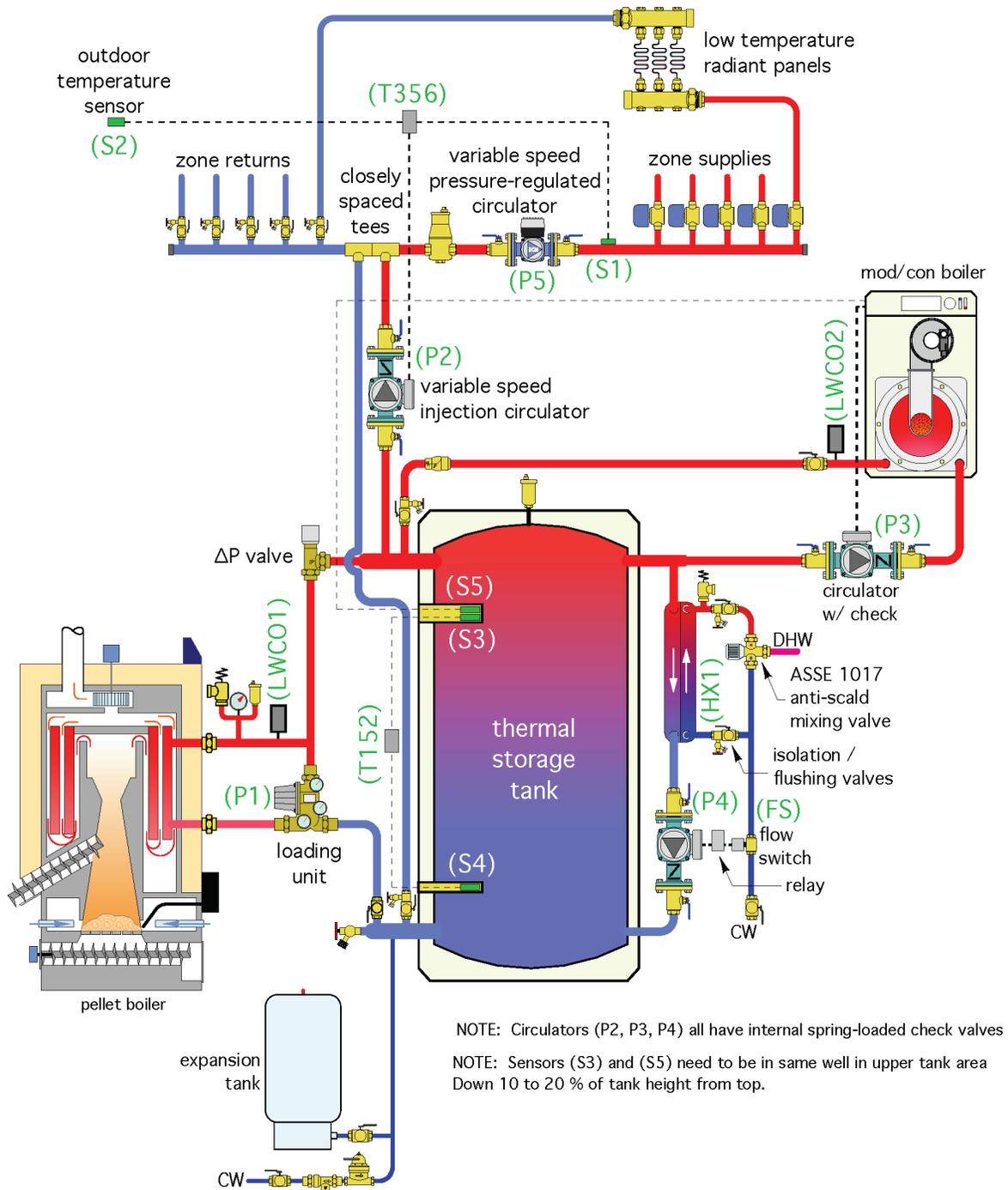
Note: Sensor (S5) should be mounted in the same well as sensor (S3). That well should be 10–20% of the tank height down from top.
