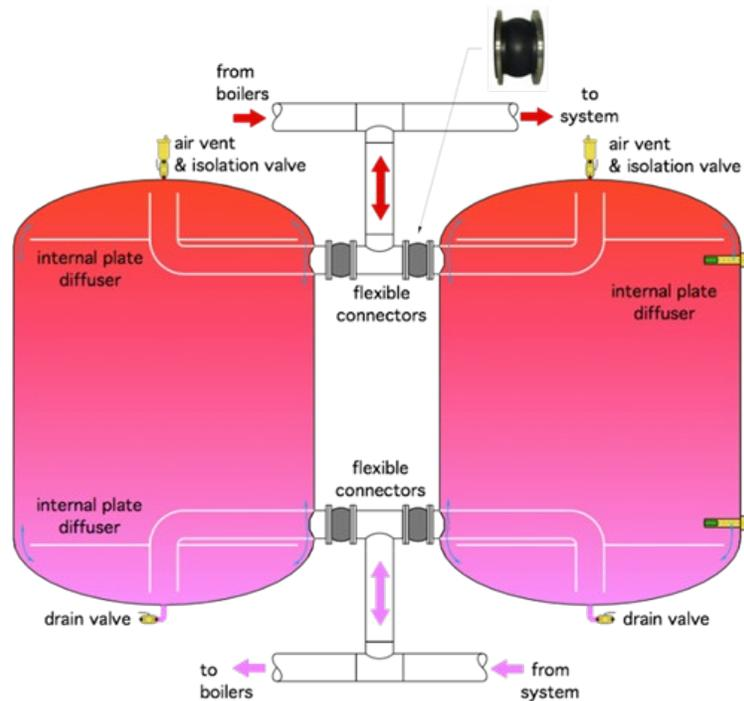
The large tanks in Figure 5-28 each have flanges at their two main sidewall connections. Threaded openings are provided for small piping, valves, or instrument.
