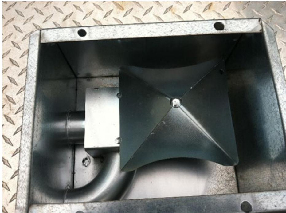
The receiver reduces weight-induced packing of pellets, allowing them to be freely entrained by a fast-moving air stream and carried from the receiver to the day hopper. The pyramid shaped baffle in the receiver creates a space beneath the pellet column where the suction effect created by a fast-moving air stream can entrain pellets, carrying them into the supply tubing.
