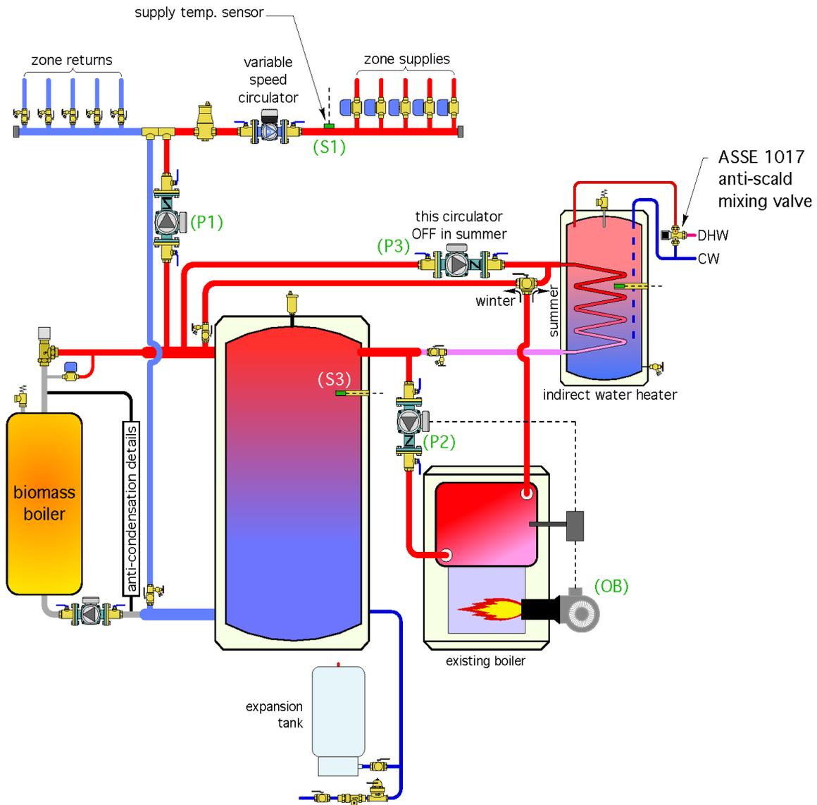
This system allows the existing/auxiliary boiler to provide supplemental heat for space heating and domestic water heating during the heating season. It also allows the existing/auxiliary boiler to supply heat directly to the indirect water heater if the pellet boiler is turned off during warm weather. Doing so reduces standby heat loss from the thermal storage tank during non-space heating months.
