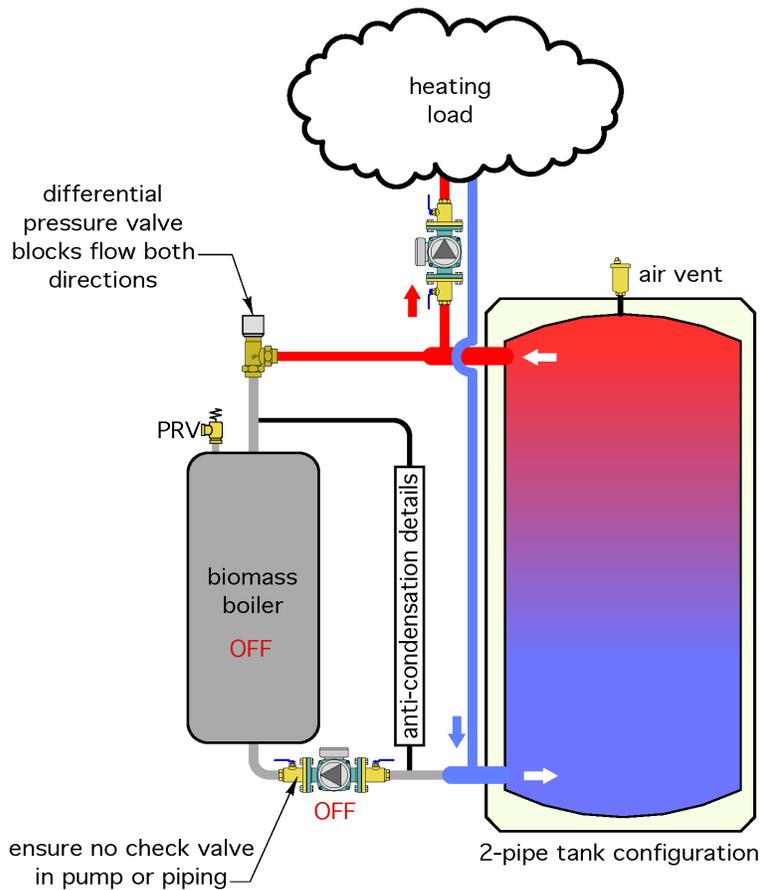
The differential pressure valve can be set to a low forward opening pressure in the range of 1–1.5 psi. This provides sufficient blocking force to prevent flow returning from the load from passing through the boiler when the boiler circulator is off. When the boiler circulator turns on, it immediately creates sufficient pressure to open the  $\Delta P$  valve. Most differential pressure valves have a relatively flat  $\Delta P$  versus flow rate curve, as shown in Figure 5-20.
