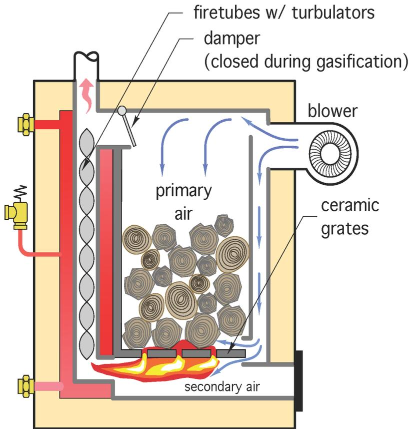
The fire in cordwood gasification boilers is started by loading smaller pieces of kindling wood at the base of the boiler's upper combustion chamber. That material is ignited and allowed to burn for a few minutes to establish a bed of hot coals at the base of the upper chamber. Then, unlike a wood stove, the upper chamber is fully loaded with firewood.
