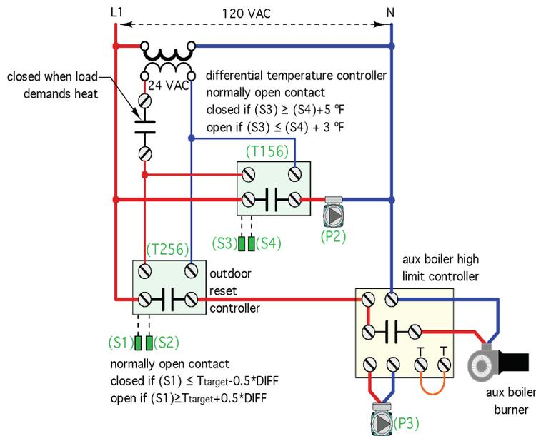
This circuitry assumes that the differential temperature controller (T156) and outdoor reset controller (T256) are powered by 24 VAC. That power only reaches both controllers when there is a heating demand in the system, which is evidenced by a closed relay contact. The latter is typically supplied from a multizone relay center or a thermostat if the building has only one zone.
