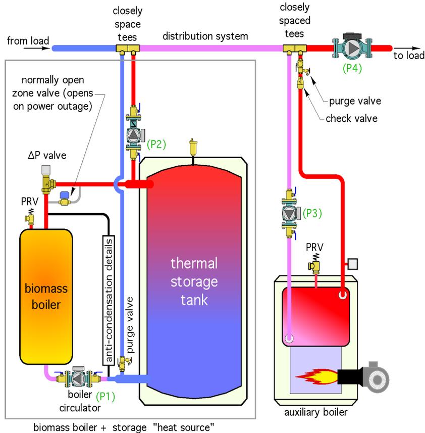
With the piping shown in Figure 7-20, heat can be supplied from the biomass boiler + storage heat source, or the existing/auxiliary boiler. Under certain conditions it's also possible to supply heat from both at the same time.
