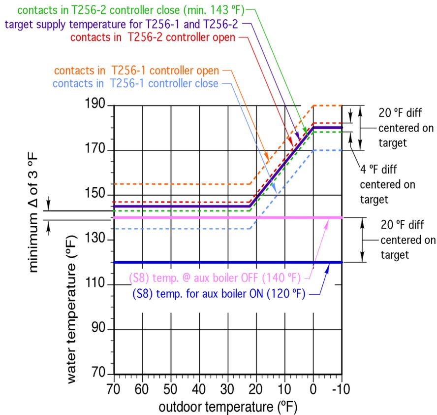
NOTE: The temperature at which the (T150-2) controller opens its contacts must be at least 3 °F lower than the lowest temperature at which the (T256-2) controller closes its contacts. In Figure 8-2c the (T150-2) controller opens its contacts at 140 °F. The lowest temperature at which the (T256-2) controller closes its contacts is 143 °F.
