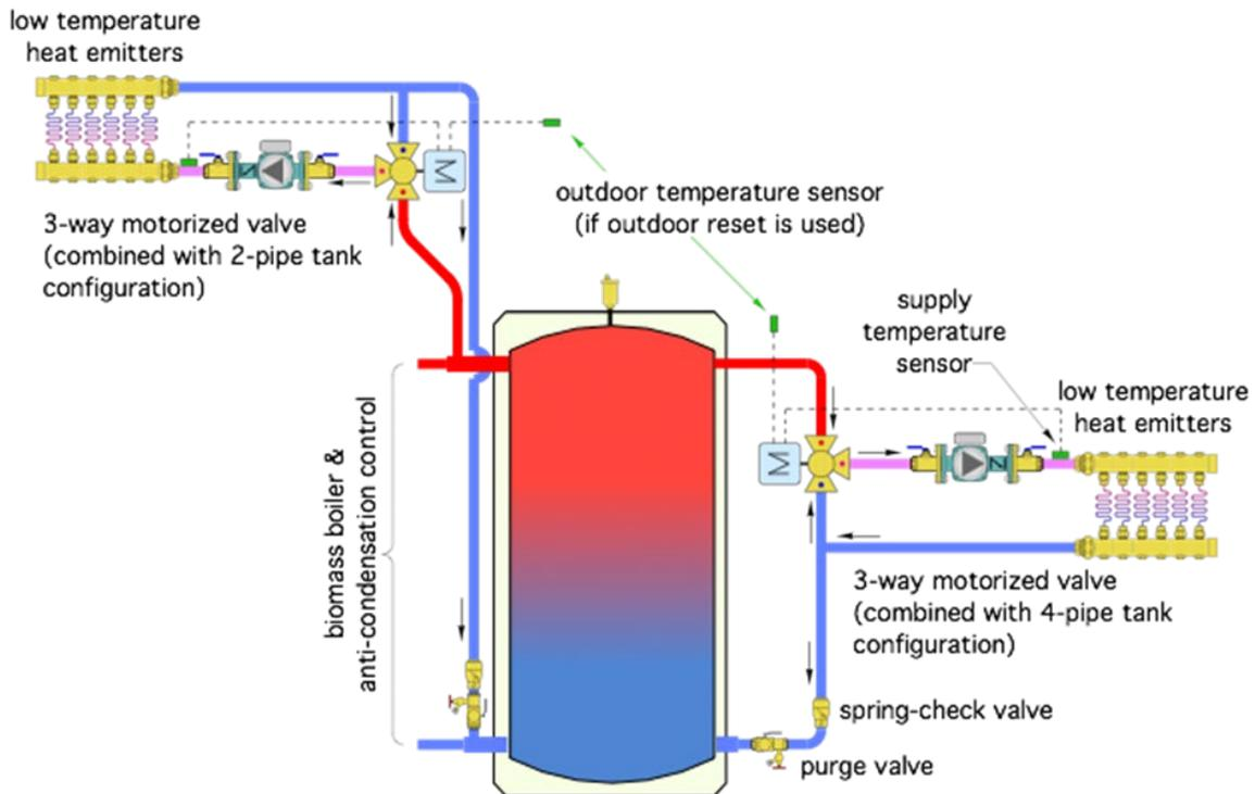
Notice that the supply temperature sensor for the controller operating the mixing valve's actuator is installed downstream of the load circulator. This ensures that the sensor detects the fully mixed water temperature on route to the heat emitters.
