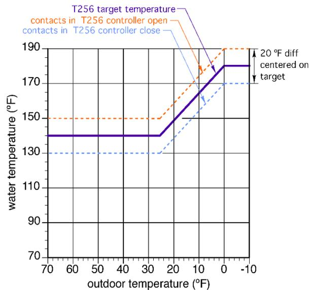
The minimum target water temperature has been limited to 140°F to prevent the oil-fired boiler from operating with sustained flue-gas condensation. If the oil-fire boiler was equipped with an anti-condensation mixing valve, the minimum water temperature could be lowered to 90°F.
