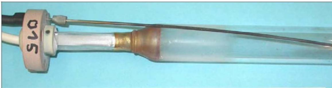
**Figure 4.46 Close up of the coated end of Type 1 MP lamp #8 on the power supply side**
