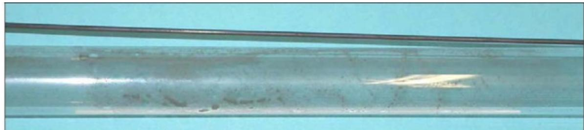
**Figure 4.45 Close up on the most fouled section of Type 1 MP lamp #8 (Position C1)**
