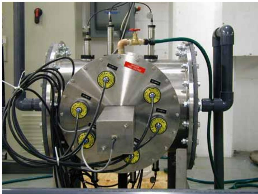
**Figure 8.3** Photograph of the IDI reactor equipped with six 6 kW MP lamps
