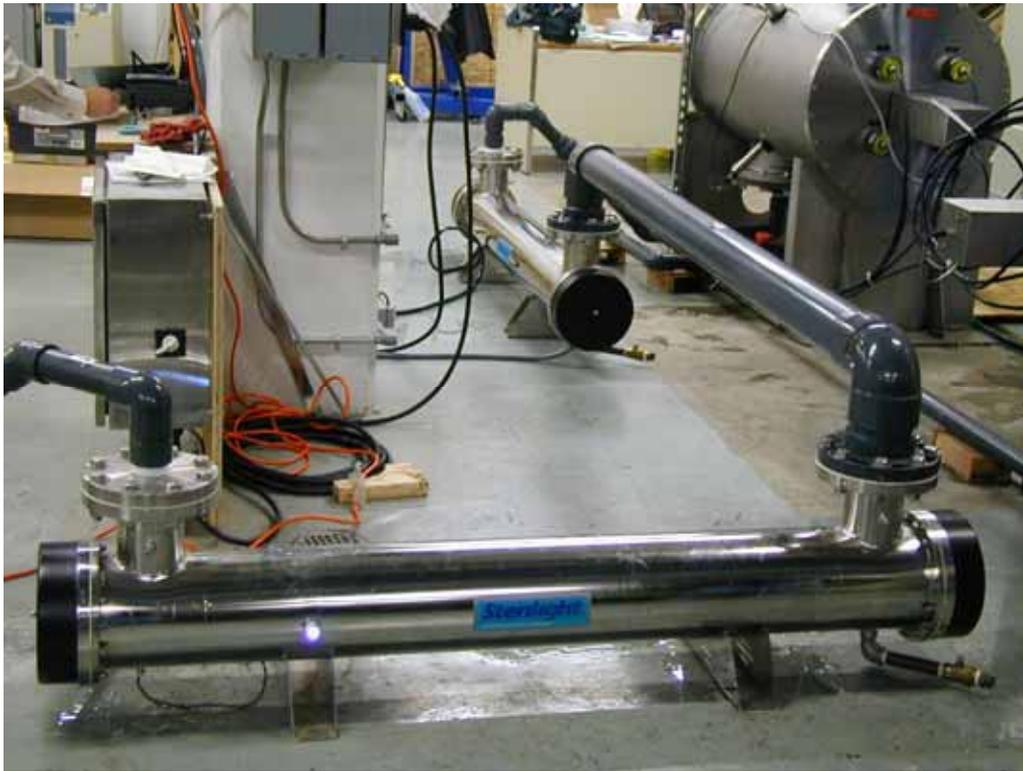
**Figure 8.2** Photograph of the R-Can amalgam and non-amalgam LPHO reactors
