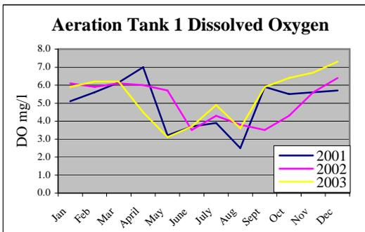
**Figure 5-3. Aeration Tank No. 1: Dissolved Oxygen**
