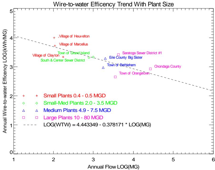
**Figure 4-3. Annual Wire-to-Water Efficiency Variation with Annual Plant Flow (Logarithmic Data)**
