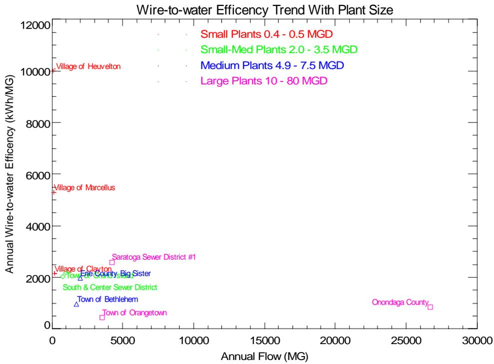
**Figure 4-2. Annual Wire-to-Water Efficiency Variation with Annual Plant Flow**
