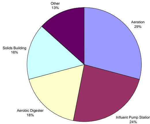
**Figure 3-10. Erie County Big Sister Creek WWTP Energy Use Breakdown**
