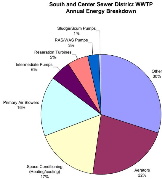
**Figure 3-7. South & Center Sewer District WWTP Energy Use Breakdown**
