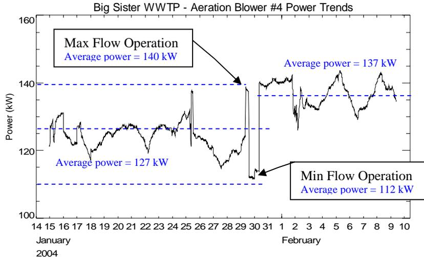
**Figure 5-5. Blower Throttling Energy Savings**
