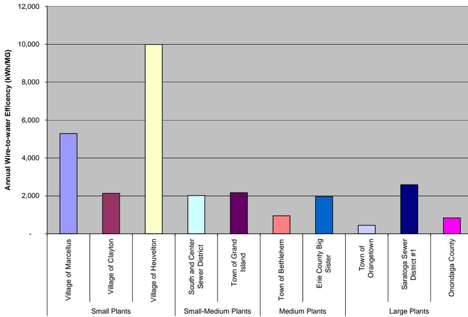
**Figure 4-1. Annual Wire-to-Water Efficiency**
