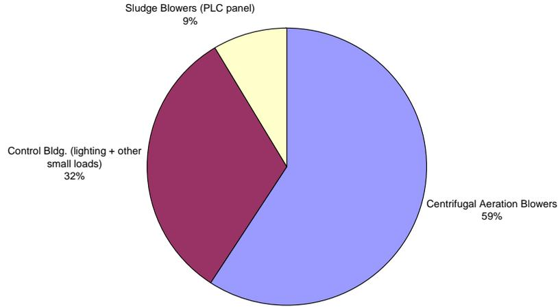
**Figure 3-5. Village of Clayton WWTP Energy Use Breakdown**
