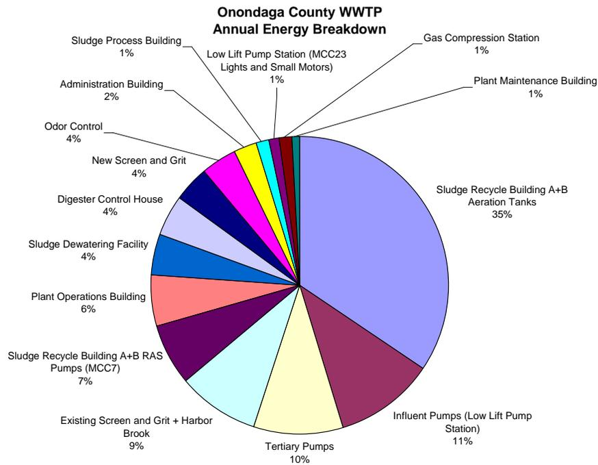
**Figure 3-13. Onondaga County WWTP Energy Use Breakdown**
