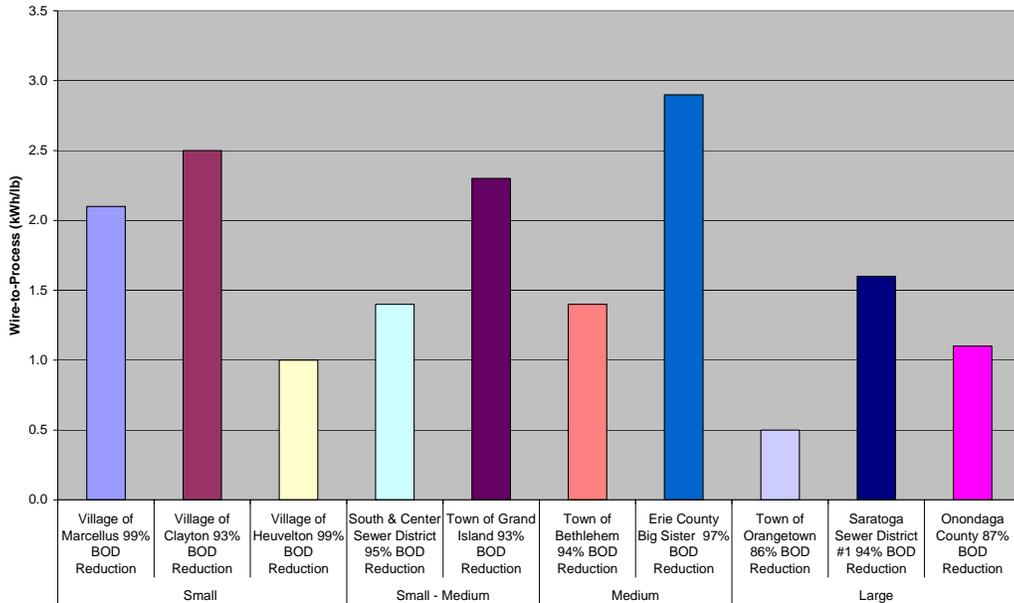
Figure 4-5. Comparing BOD Removal Energy Across all Sites (Wire-to-Process)
