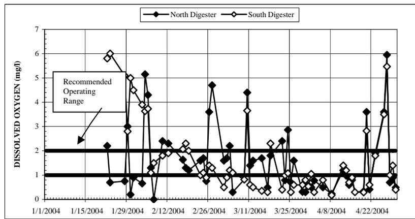
**Figure 5-7. Digester Dissolved Oxygen Concentrations**
