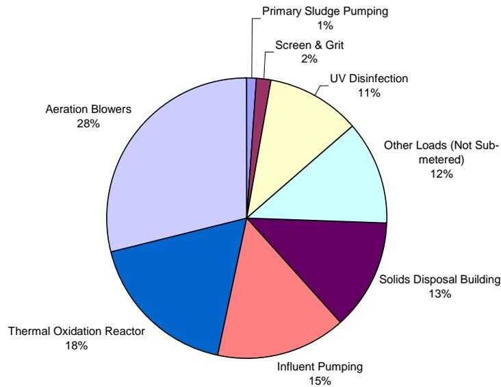
**Figure 3-12. Saratoga Sewer District #1 WWTP Energy Use Breakdown**
