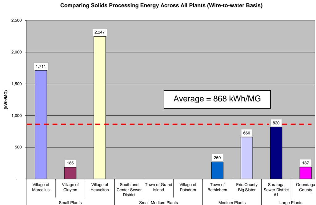
**Figure 3-18. Comparing Bio-Solids Processing Energy Across all Sites (Wire-to-Water)**
