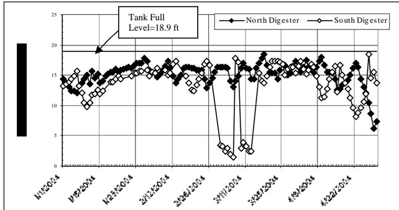
**Figure 5-6. Digester Tank Levels**
