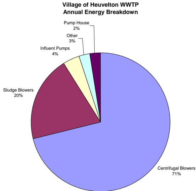
**Figure 3-6. Village of Heuvelton WWTP Energy Use Breakdown**
