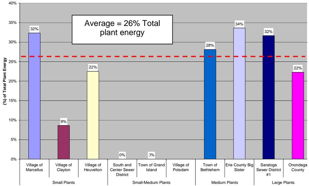
**Figure 3-19. Comparing Solids Processing Energy Across all Sites (% of Total Plant Energy)**
