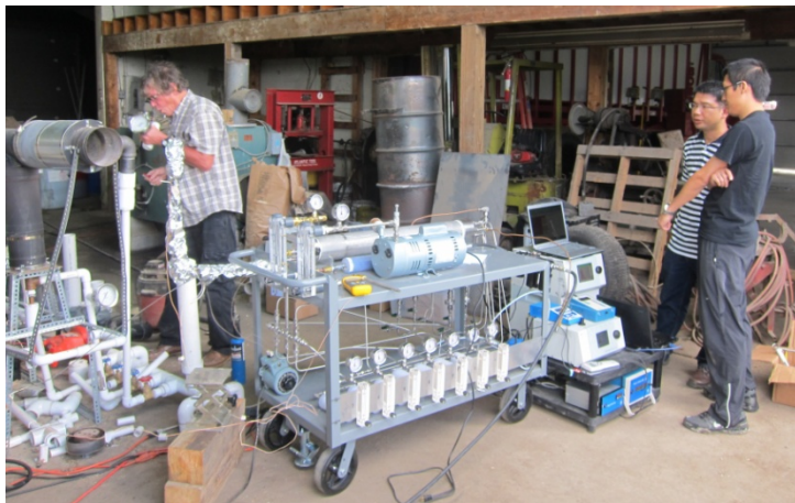
Figure 8: Experimental setup for the wood power burner in King Ferry, N.Y.
