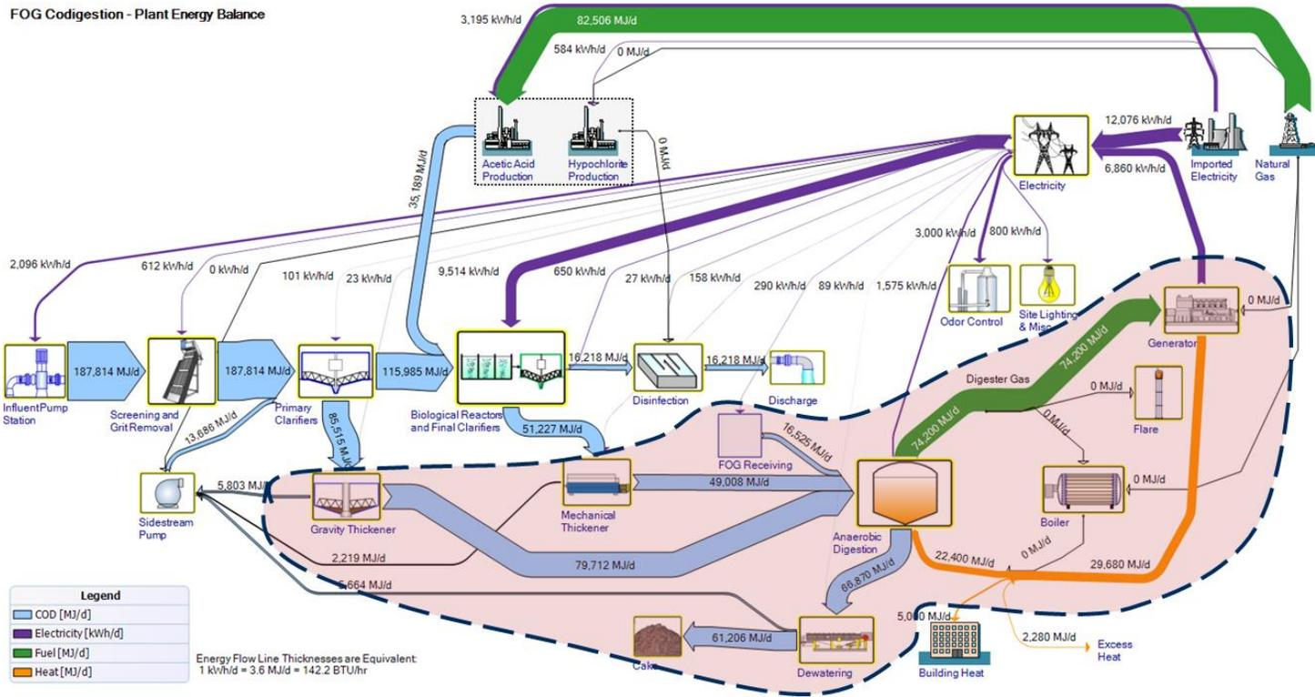
**Figure 3-2. Sankey Diagram for Configuration 2X/2Y, Scenarios with Activated Solids with BNR, WAS Mechanical Thickening, Anaerobic Digestion with FOG Co-Digestion, Dewatering, and CHP.**
