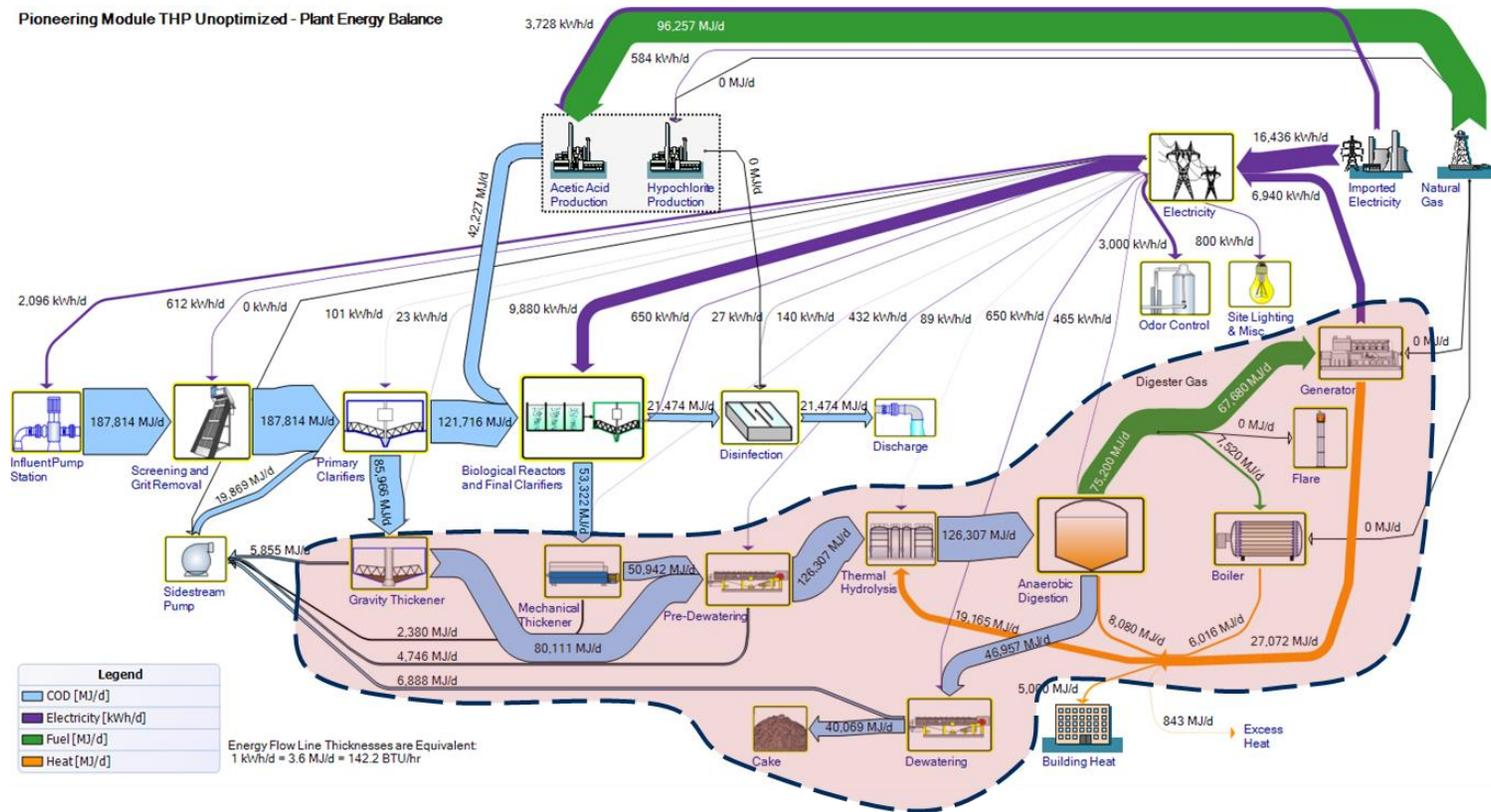
Figure 3-1. Sankey Diagram for Configuration 1X/1Y, Scenarios with Activated Solids with BNR, Pretreatment (thermal hydrolysis), WAS Mechanical Thickening, Anaerobic Digestion, Dewatering, and CHP.
