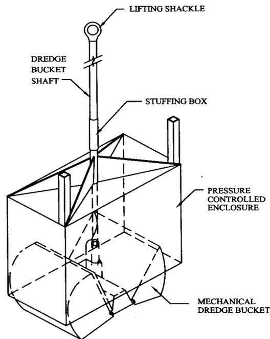
**Figure 4-1: Enclosure and Bucket**
