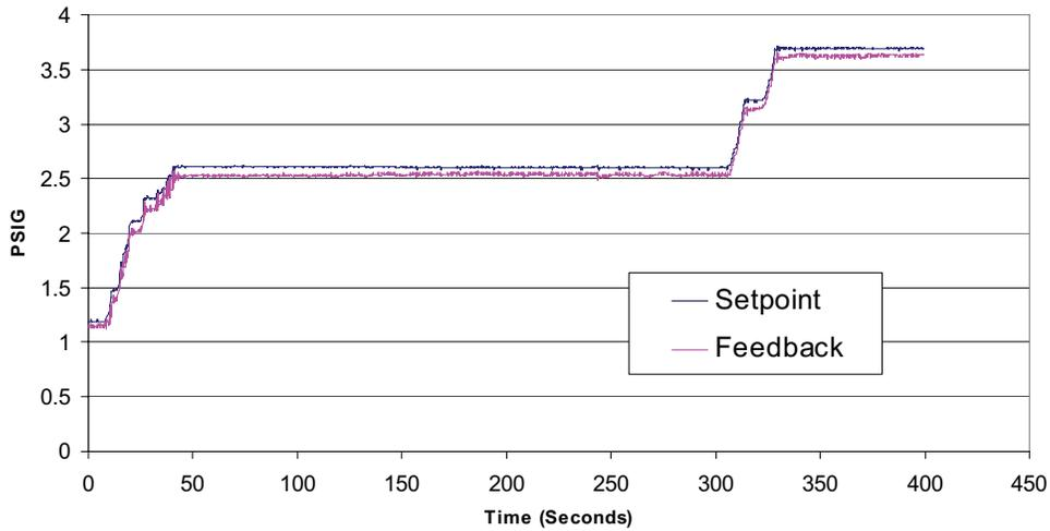
**Figure 5-20: Pressure-Controlled Excavator 12-ft Tank Test: Descending Readings**
