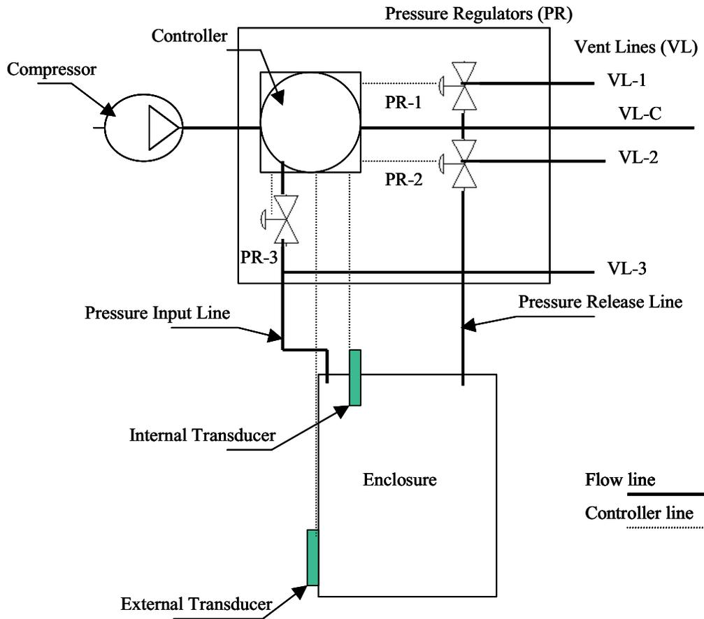
**Figure 4-4: Pressure Controller Feedback Control System**
