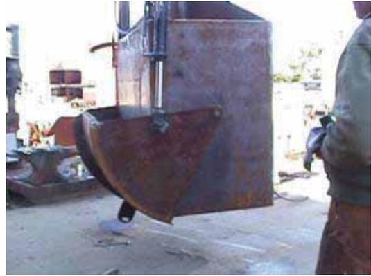
**Figure 5-8: Enclosed Excavator with Partially Closed Door**
