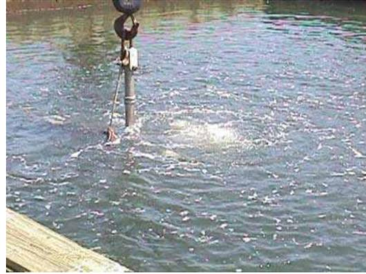
**Figure 5-27: Over-Pressurized Field Prototype**
