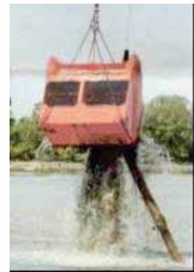
**Figure 2-3. Leaky Clamshell Buckets**
