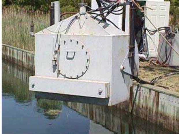
**Figure S-2: Pressure-Controlled Excavator Ready for Submersion**
