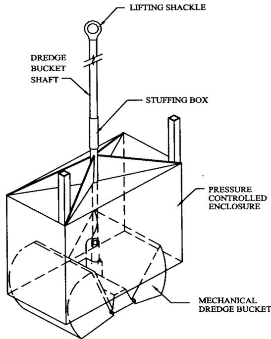
**Figure S-1: Pressure-Controlled Enclosure and Bucket**
