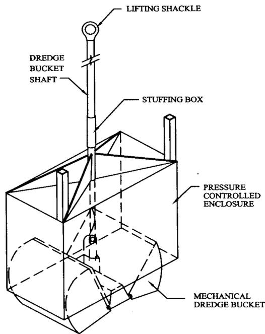
**Figure 4-1: Enclosure and Bucket**
