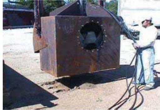
**Figure 5-10: Enclosed Excavator Maintenance Hatch**
