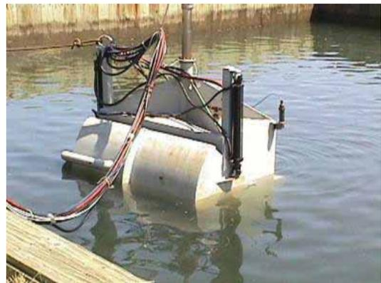
**Figure 5-25: Field Prototype Unit Descending for Excavation**
