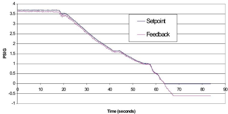
**Figure 5-21: Pressure-Controlled Excavator 12-ft Tank Test: Ascending Readings**
