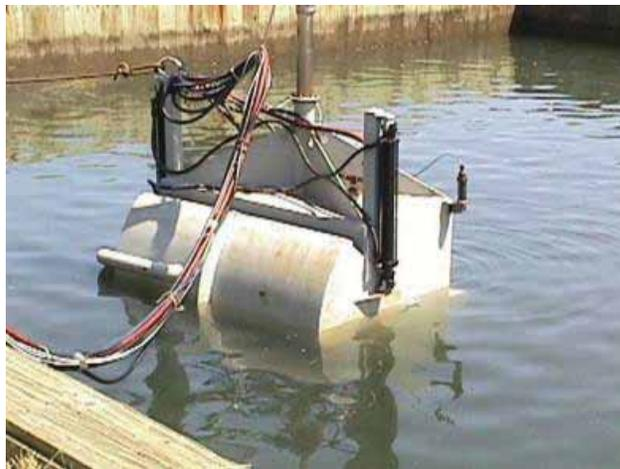
**Figure S-3: Pressure-Controlled Excavator Descending Below Surface for Excavation**
