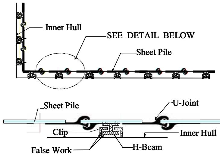
**Figure 3-5. Support Structure System Details**
