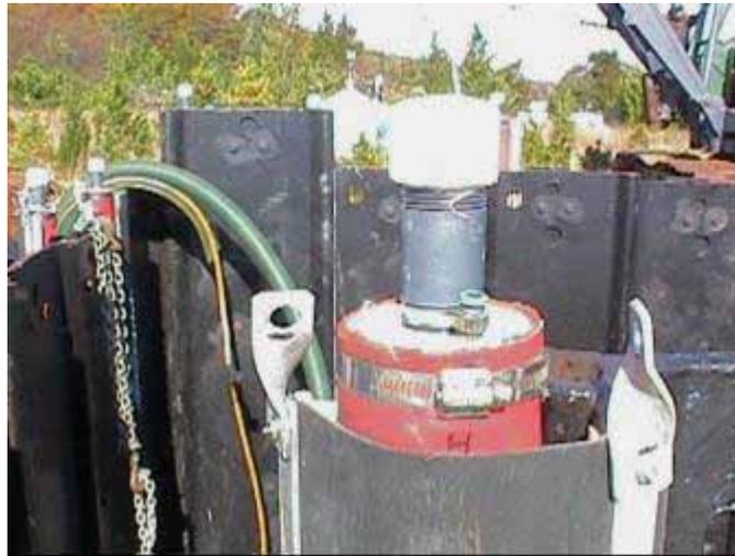
**Figure 6-3. Sealing Tube Cap and Air-Fill Port**
