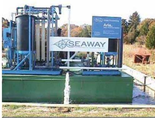
**Figure 4-1. Mobile Water Filtration Plant
