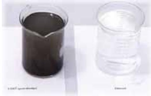
**Figure 4-3. Mobile Water Filtration Plant Results (Influent Water On Left and Effluent on Right)**
