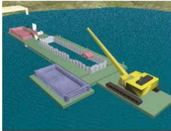
**Figure 4-5. Mobile Containment Vessel and Mobile Water Treatment Vessel Deployment**
