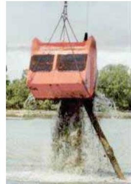
**Figure 2-3. Leaky Clamshell Buckets**
