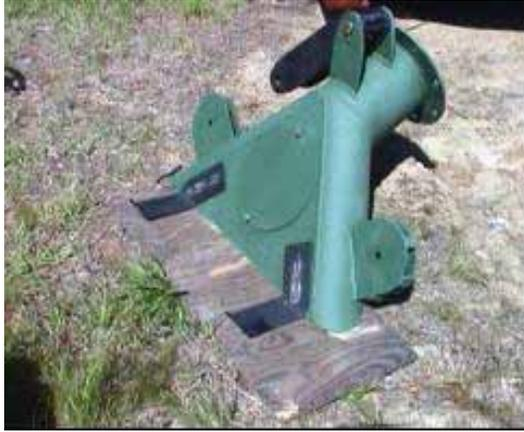
**Figure 4-4. Cutter-less Vacuum Head**
