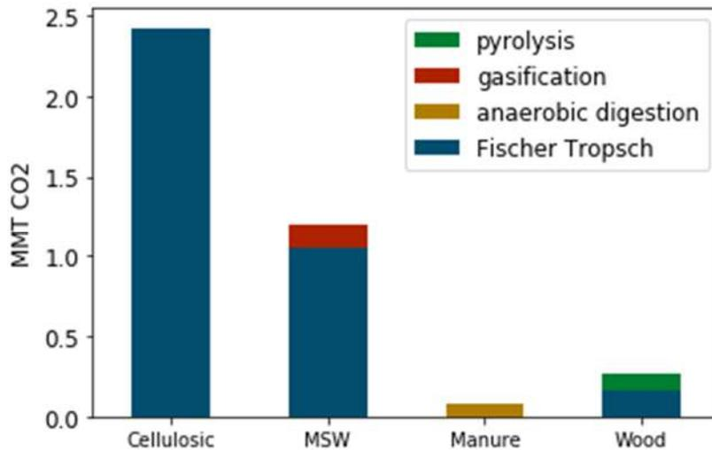
**Source:** E3 analysis of potential carbon abatement of in-state MSW and agricultural feedstock from federal report<sup>25</sup> on biomass feedstocks, and additional landfill gas and WWTP feedstock from NYSERDA report.<sup>26</sup>
