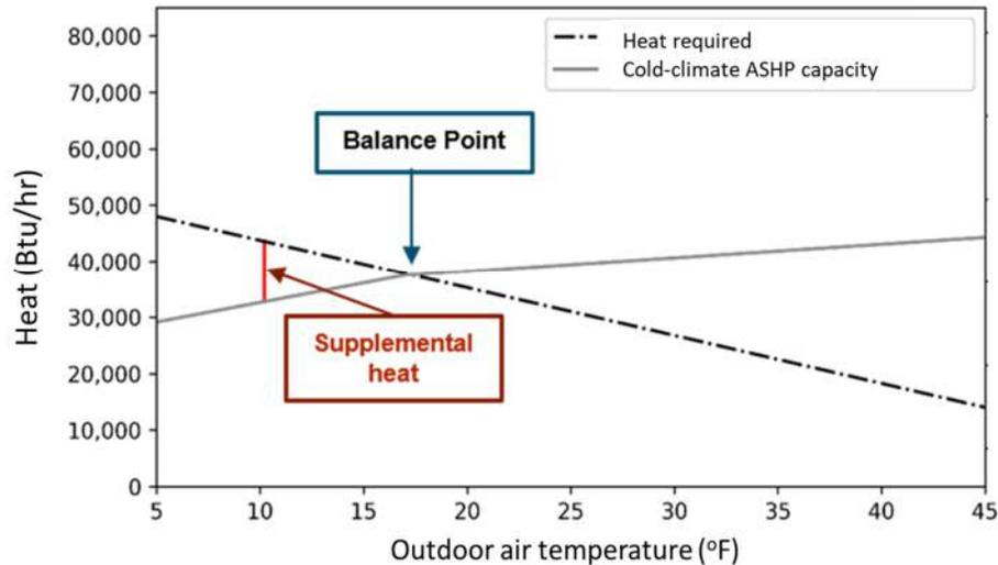
**Source:** E3 RESHAPE analysis of example cold climate ASHP output as function of outdoor air temperature in home which demands 48 kBtu/hr of heat at air temperature of 5°F.
