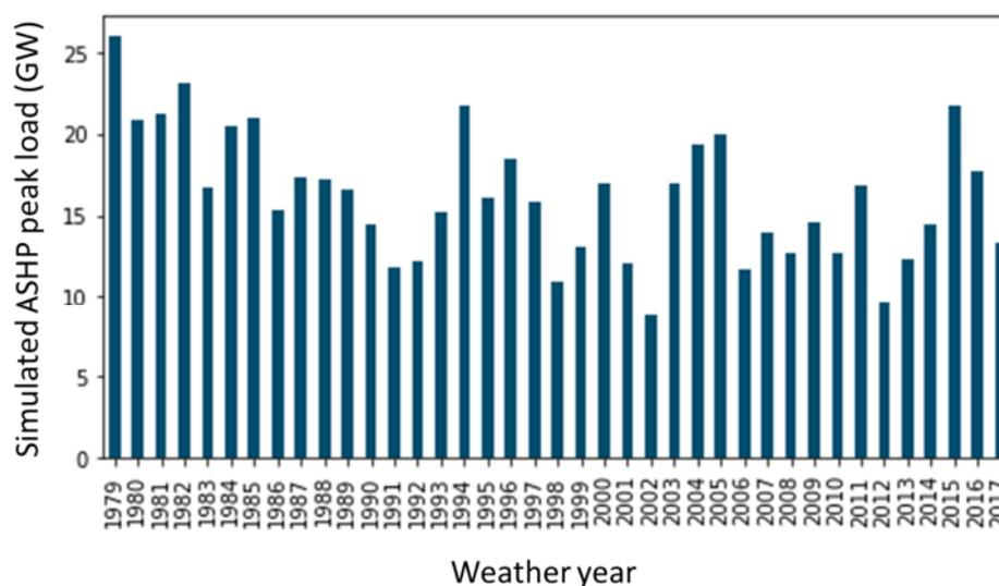
**Source:** E3 RESHAPE analysis to simulate potential ASHP peak loads under Decarbonization Pathways scenario levels of heat pump market penetration in 2050, using 1979-2017 weather year data and assumptions on heat pump efficiency, building shell improvement, supplemental heat source, and heat pump sizing as discussed above.
