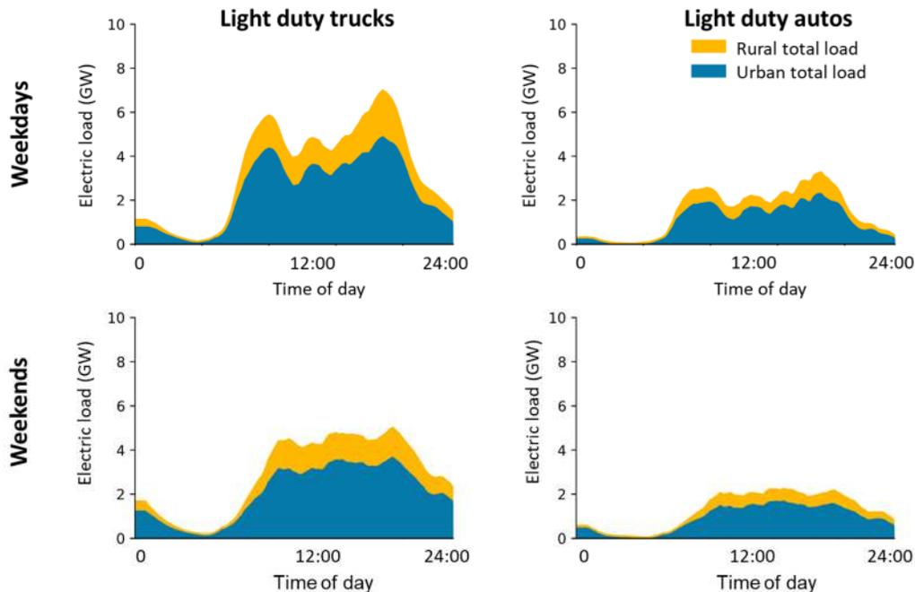
**Source:** E3 analysis of sample weekday and weekend vehicle charging profiles for example urban and rural locations in New York State assuming 100% electric vehicle market penetration. These load shapes are representative, and the magnitude of the true electric vehicle load shape would depend on the market penetration of electric vehicles simulated in each region.
