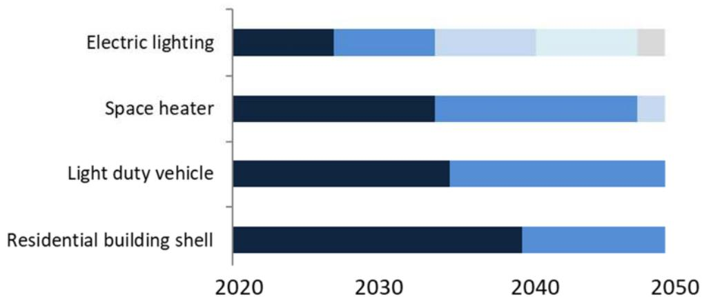
**Source:** Illustrative data. Each color represents a stock rollover point in which a technology retires and is replaced with a new one. Note shorter lived technologies, such as, roll over multiple times whereas longer lived technologies, such as building shell, roll over only once in this graphic.
