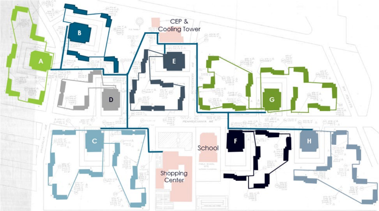
Figure 1. Spring Creek Towers Central Energy Plant and Thermal Distribution Networks
