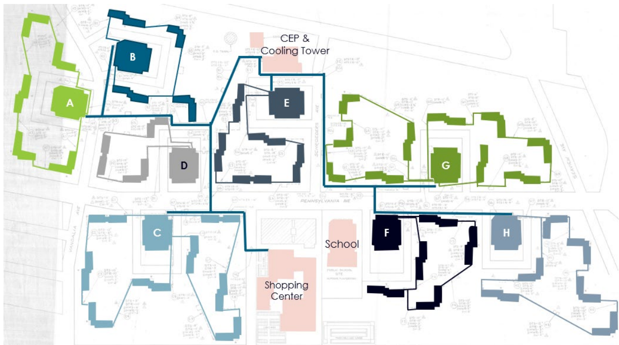
Figure A-1. Central Energy Plant, Primary Distribution Garages, and Secondary Distribution Loops
