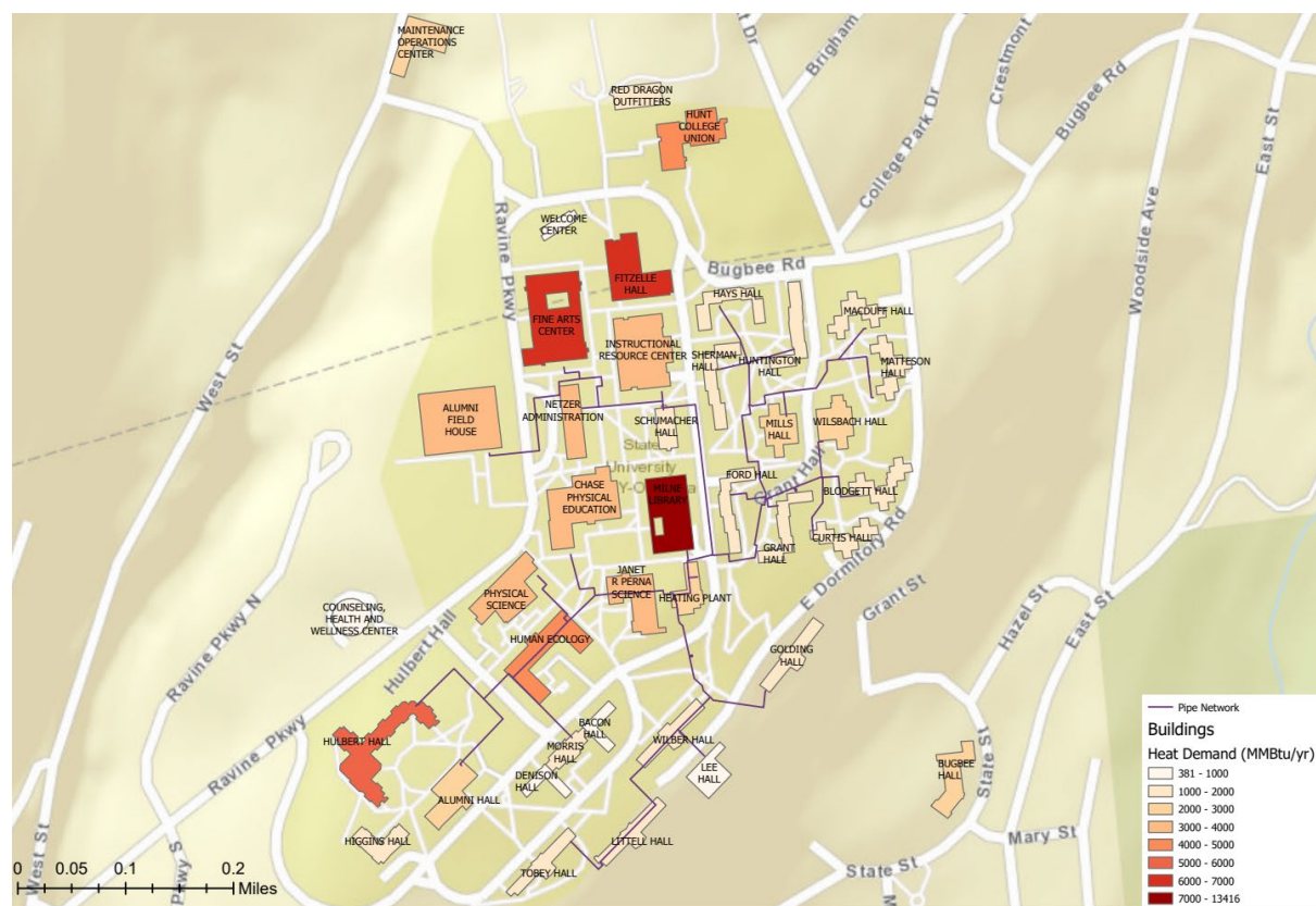
Figure 14. Heat Mapping of SUNY Oneonta in ArcGIS
