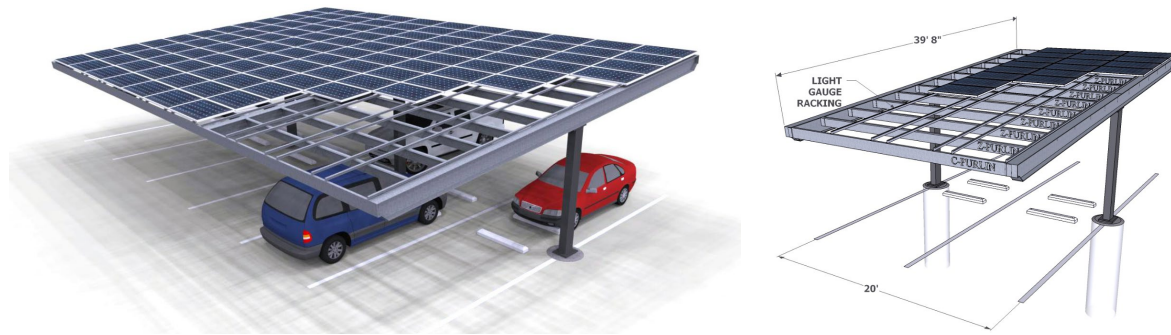
Figure 31. Single-Column, Double-Style Carports
