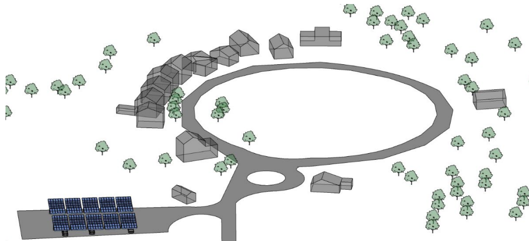
Figure 30. 176-kilowatt Carport Solar Array on Existing Parking Lot
