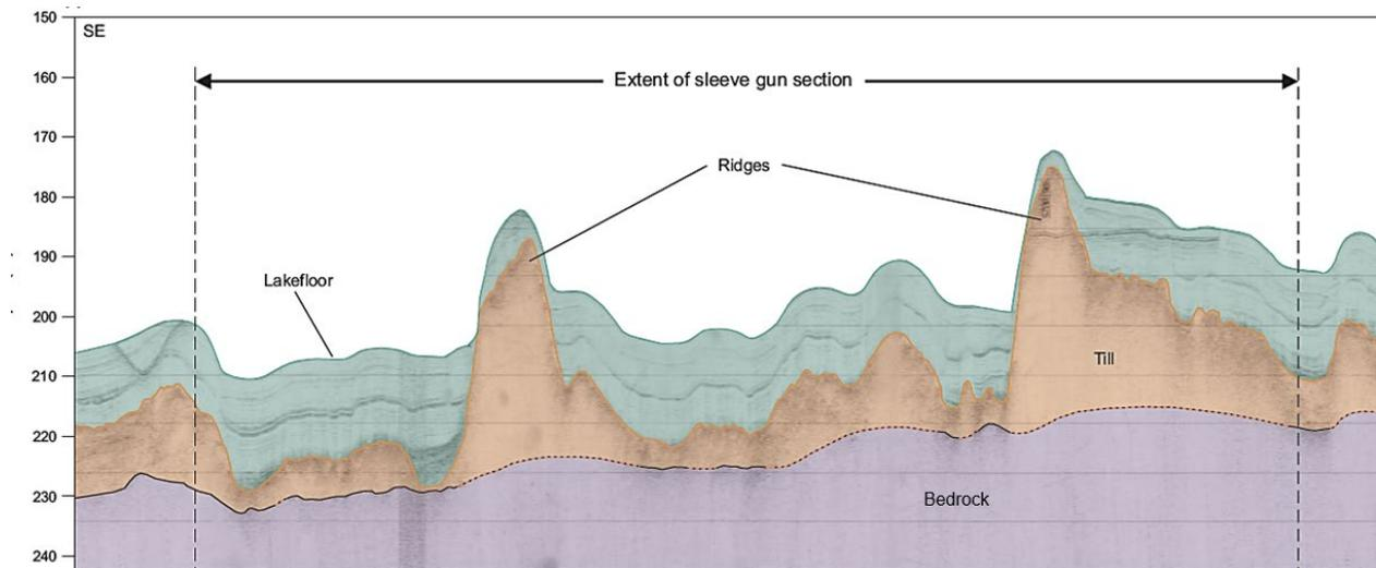
In this cross-section, the water depth varies between 175 and 210 meters in the middle of Lake Ontario between the ports of Oswego and Rochester. Careful consideration would need to be taken for how a mooring system would interact with the lakebed at a specific site in the presence of these geotechnical obstacles, and they may prohibit anchor placement in some areas. Because the presence of these drumlins is deterministic, they can be avoided with proper siting.
