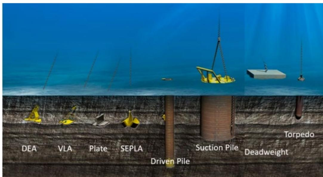
The specific anchor selection for a mooring system depends on a multitude of factors, including the floating substructure type, the substructure's compatibility with a mooring system, the mooring configuration, soil conditions, the expected embedment depth, mooring line tensions, the anchor holding capacity, installation plans, and cost. The following describes common anchors in more detail.
