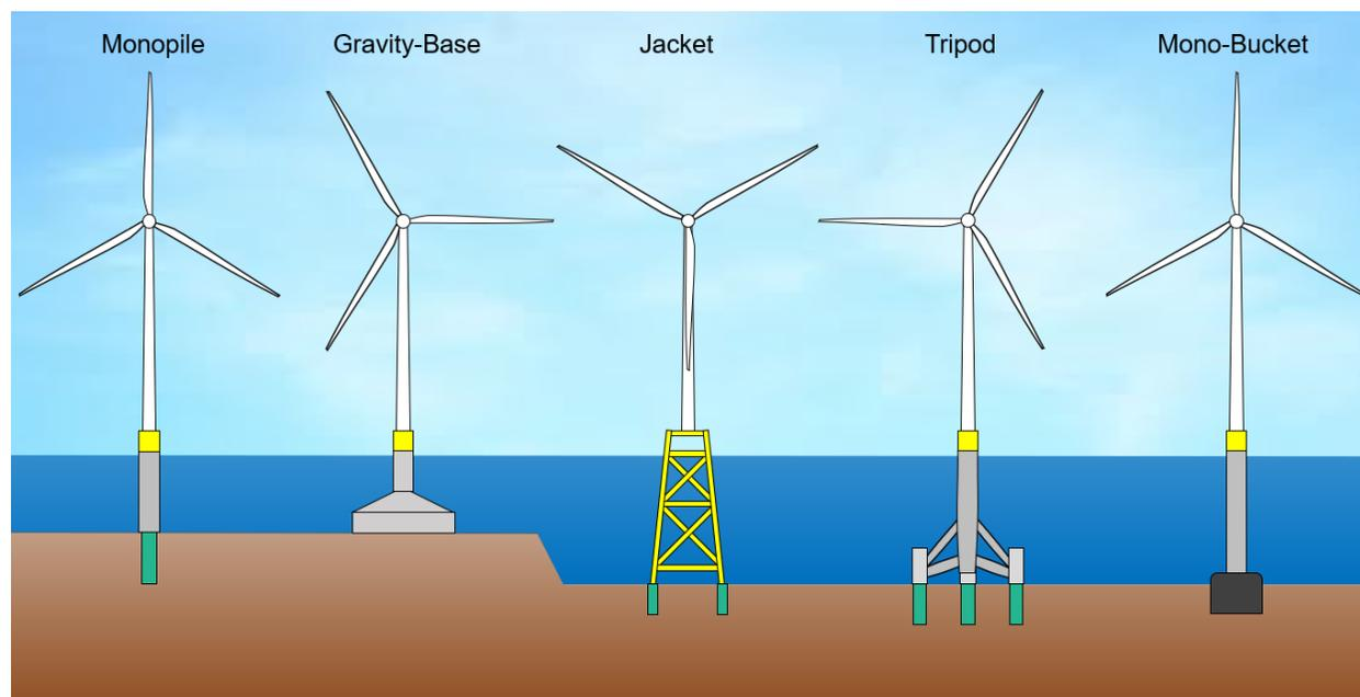
Great Lakes Wind (GLW) would likely deploy similar types of fixed-bottom substructures as Figure 1, but the designs would require modifications to accommodate the physical and logistical conditions of the Great Lakes. Primary examples of these conditions include the presence of freshwater ice, differing soil properties and strengths, and the restricted availability of heavy lift vessels for installation.
