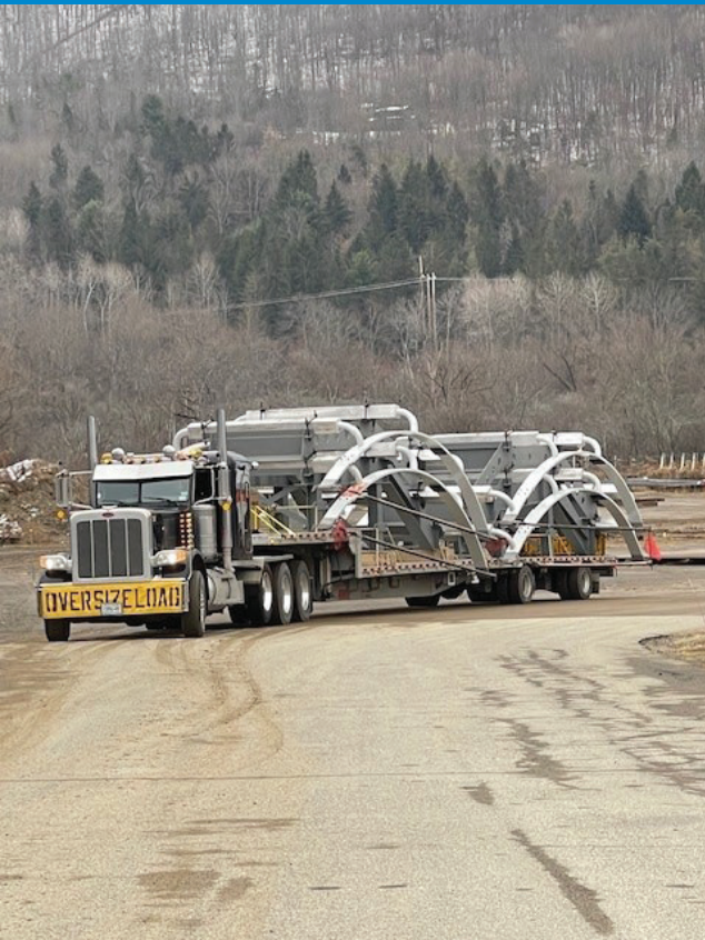
Anode Cage: Dimensions differ depending on the foundation of a turbine but the component is scaling to 37' in diameter x 14' in height and weighing 21 tons (42,000 lbs) and protect steel foundations from corroding under the conditions of the ocean.
