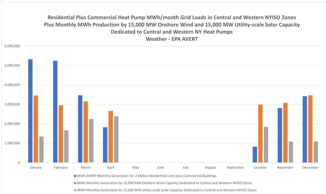
Figure 19. Monthly Grid Loads plus 15,000 MW Wind Capacity plus 15,000 Solar Capacity – Central and Western NYISO Zones
