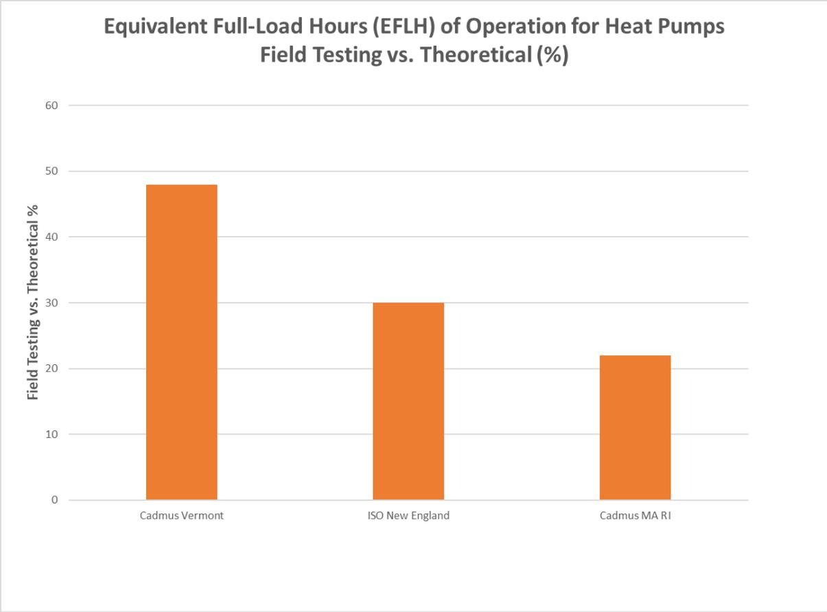
Figure 3. Equivalent Full-load Hours of Operation for Heat Pumps – Field Testing vs. Theoretical (%)
