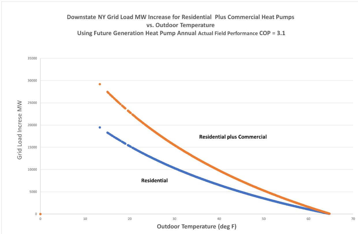
Figure 16. Grid Load Increase (MW) vs. Outdoor Temperature for Full Implementation of Residential and Commercial Heat Pumps in Downstate NYISO Zones
