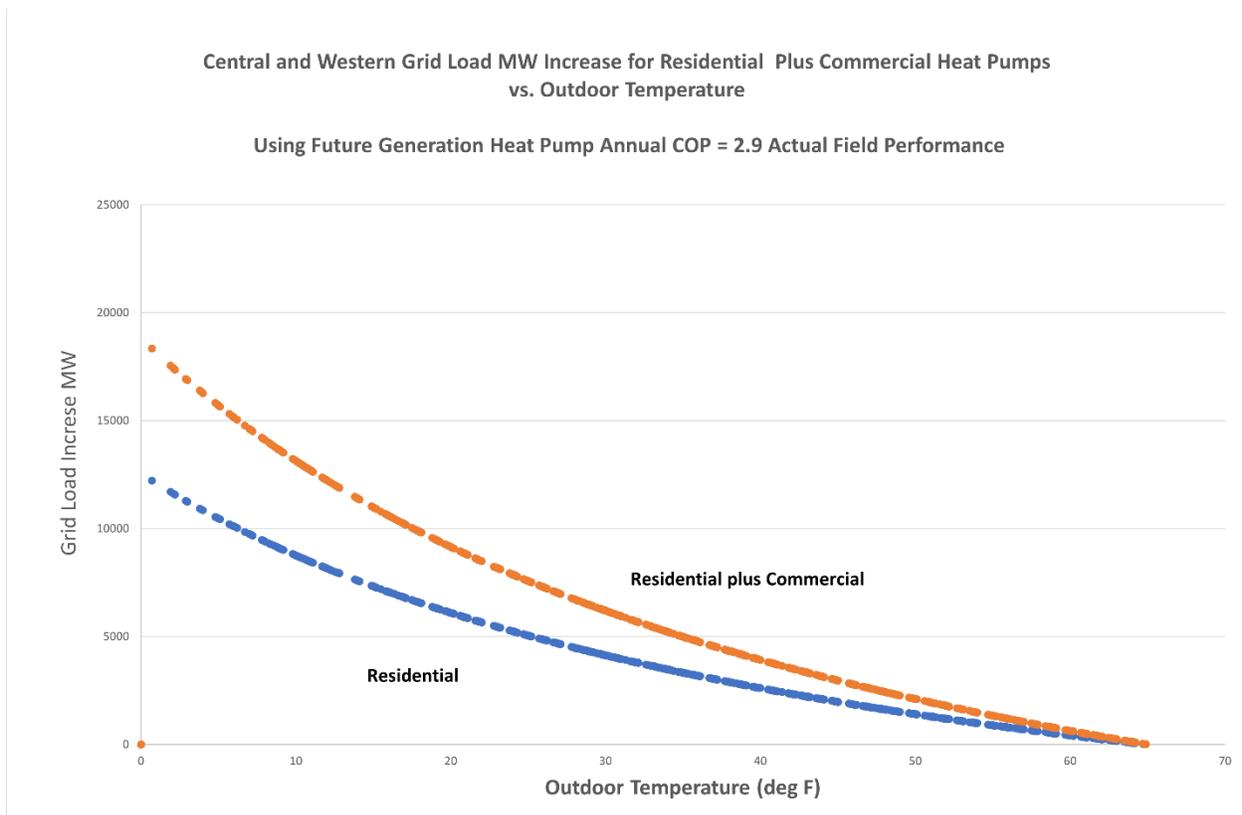
Figure 17. Grid Load Increase (MW) vs. Outdoor Temperature for Full Implementation of Residential and Commercial Heat Pumps in Central and Western NYISO Zones
