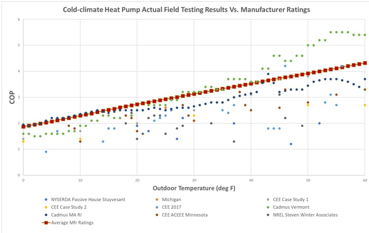
Figure 20. Cold-climate Heat Pump Actual Field Testing Results vs. Manufacturer Ratings
