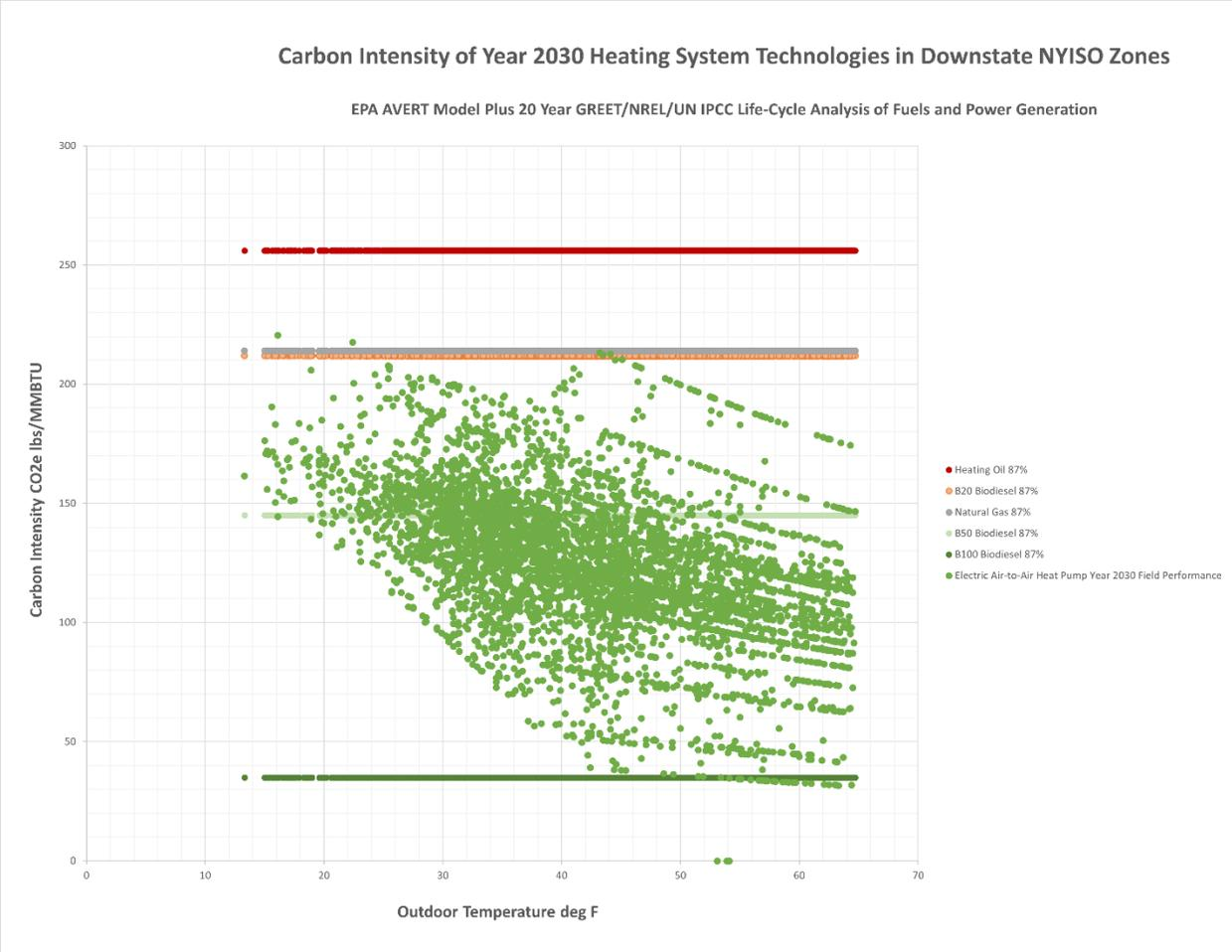
Figure 14. Existing, Time-weighted, Carbon Intensity (lbs CO<sub>2</sub>e per MMBTU) vs. Outdoor Temperature for Year 2030 Heating Technologies in Downstate NYISO Zones
