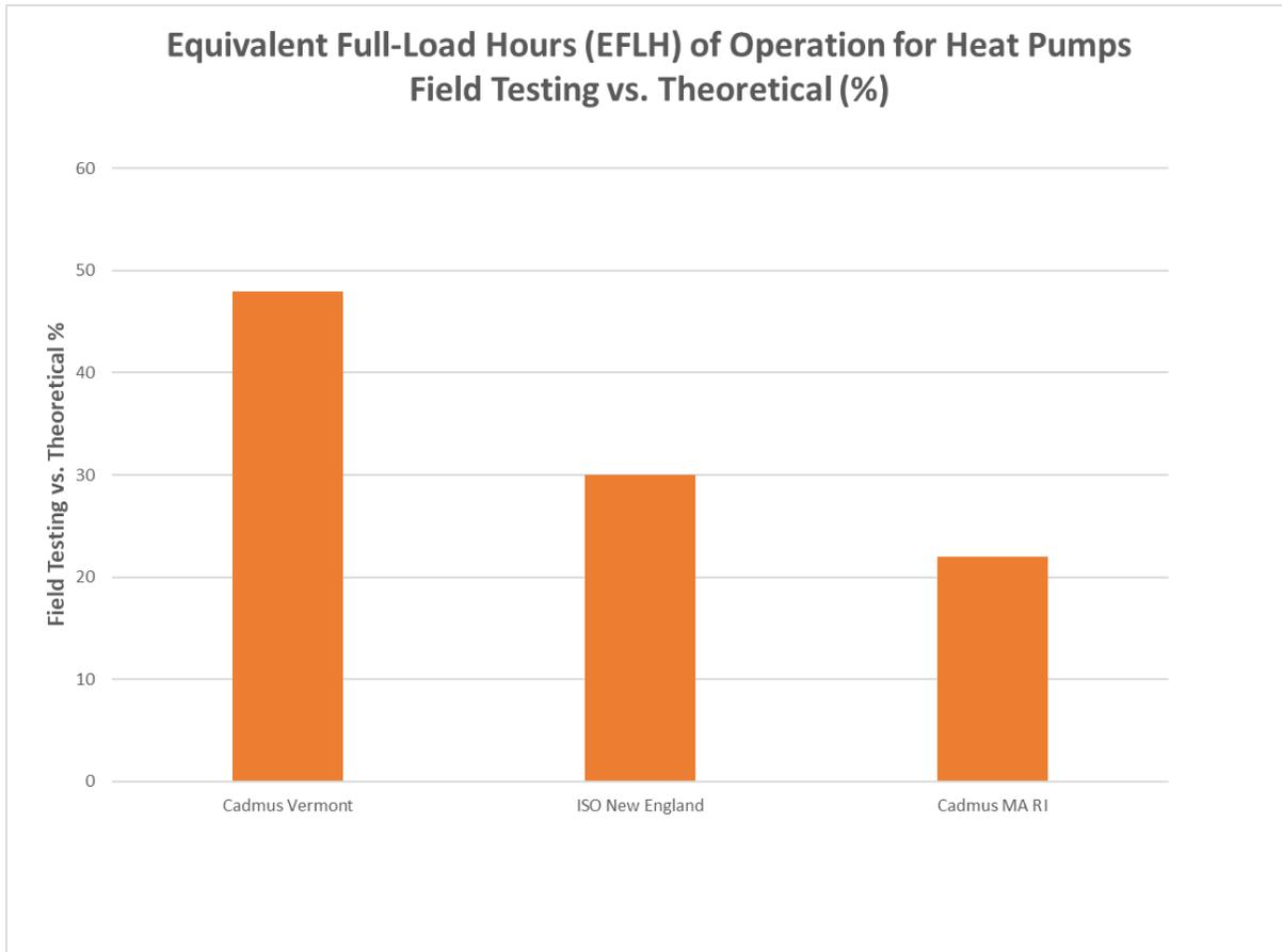
Figure 23. Equivalent Full-Load Hours of Operation for Heat Pumps
