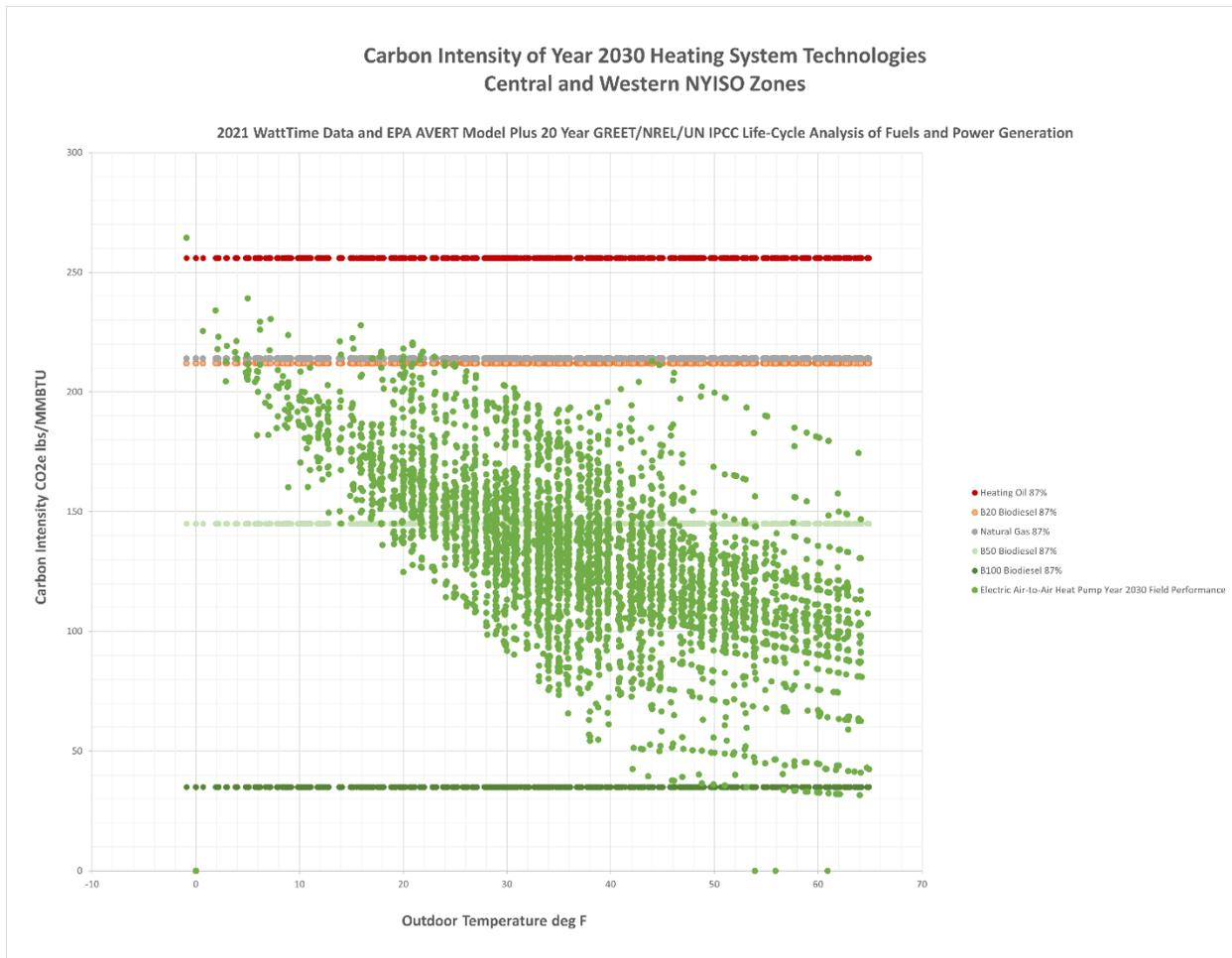
Figure 15. Existing, Time-weighted, Carbon Intensity (lbs CO<sub>2</sub>e per MMBTU) vs. Outdoor Temperature for Year 2030 Heating Technologies in Central and Western NYISO Zones
