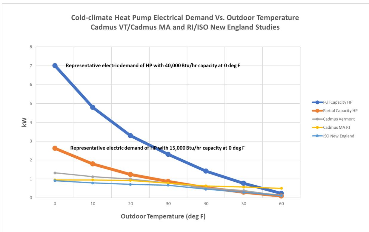
Figure 22. Cold-climate Heat Pump Electrical Demand vs. Outdoor Temperature
