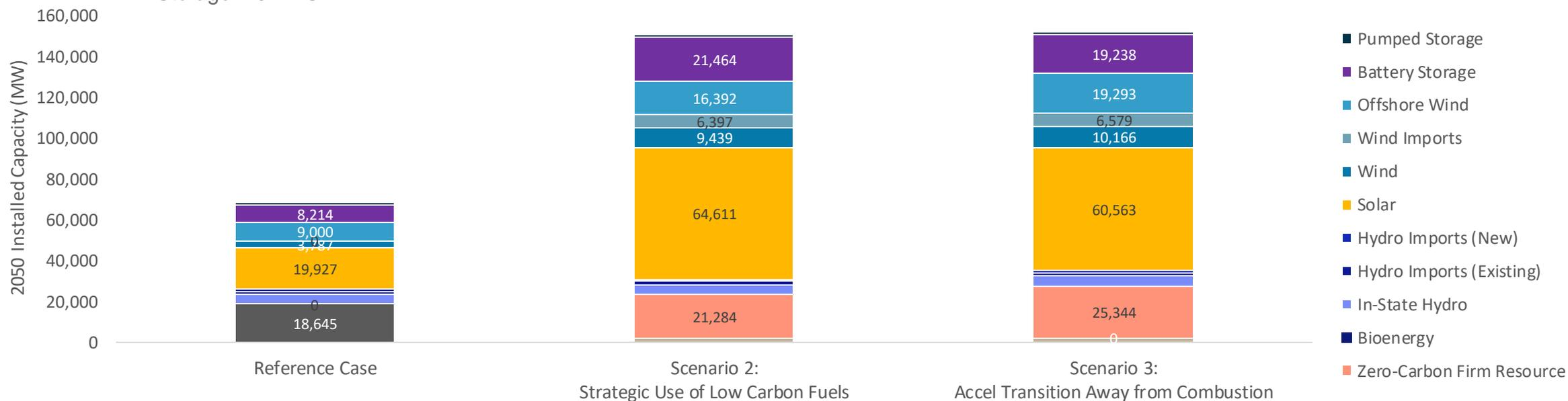
Note: In Scenario 3, existing fossil fuel resources are retired by 2040 and no new combustion-based (CCGT or CT) capacity is permitted. New firm capacity is provided by a combustion-free resource (e.g. hydrogen fuel cells).
