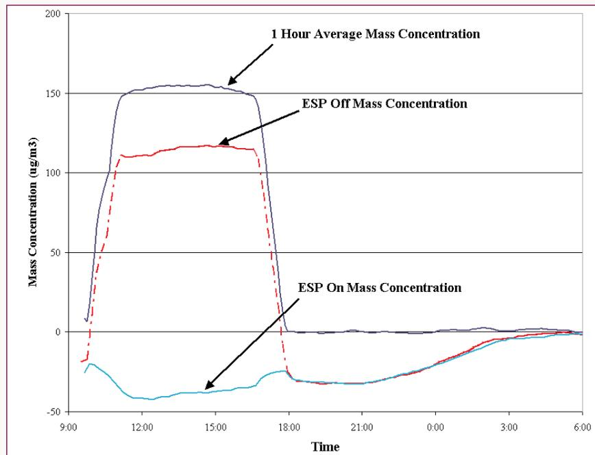
**Figure 4.** Performance of prototype Differential TEOM monitor sampling ammonium nitrate from an aerosol chamber at the Atmospheric Sciences Research Center, University at Albany, SUNY. [Measured mass concentration (red line) when ESP is on represents evaporation of ammonium nitrate from sample filter. True net mass concentration (black line) is obtained by subtracting the mass concentration when ESP is on from the mass concentration measured when ESP is off (normal collection).]
