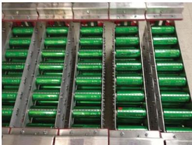
Testing is underway to use capacitors as energy storage devices on subway cars. The capacitors will absorb regenerative braking energy and then release energy to supplement acceleration.
