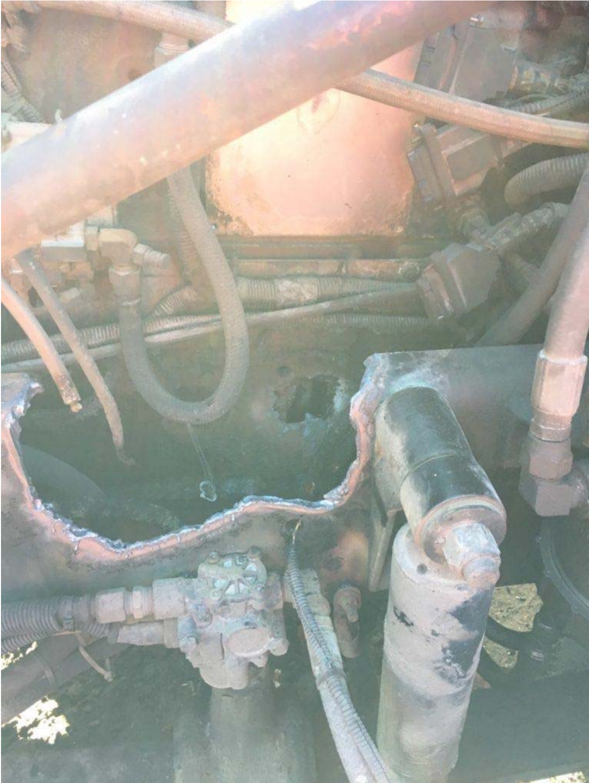
Example of complete engine hole
