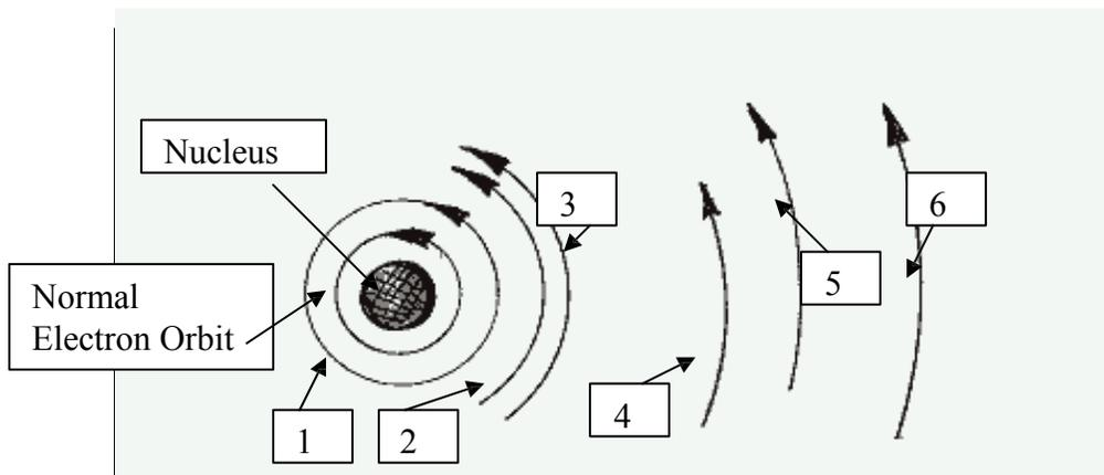
The electron remains at the higher energy level only momentarily, and then falls back toward its original normal level just like the steel ball falling to the foil.
