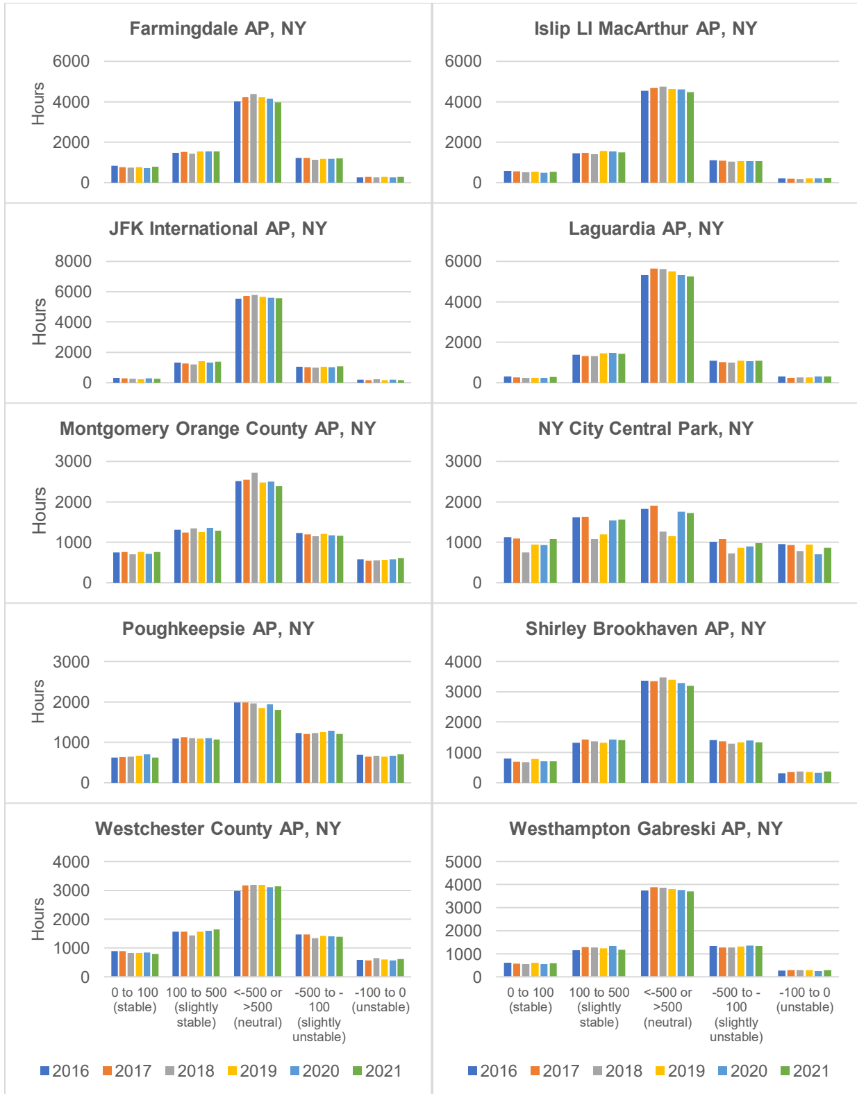
Figure A-5. Distribution of the Number of Hours per Year with Monin-Obukhov Length Values in Different Stability Ranges (Subset of Meteorological Stations in NYS, 2016-2021)
