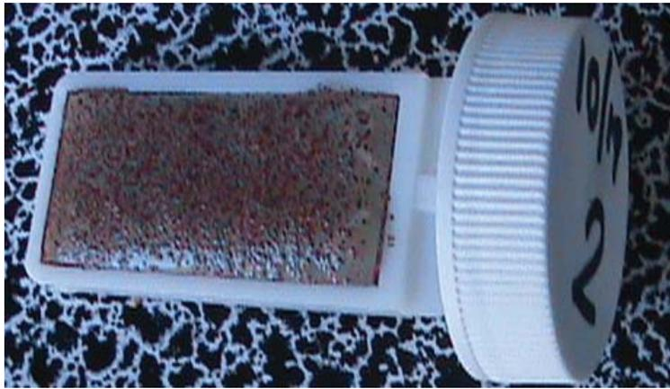
Figure 4-5. Dipslide indicating initial bacteria level.
