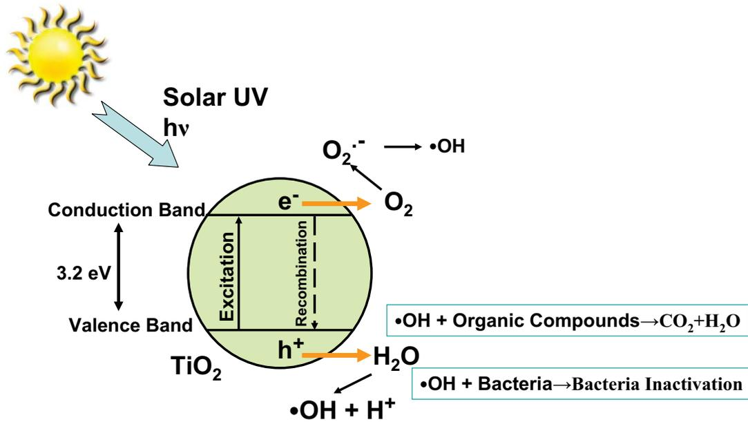
Figure 2-1. A schematic illustration of solar UVPCO mechanism.
