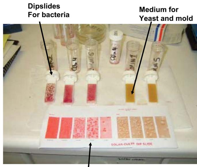
Figure 3-5. A photo illustrating bacteria testing using Dipslides.
