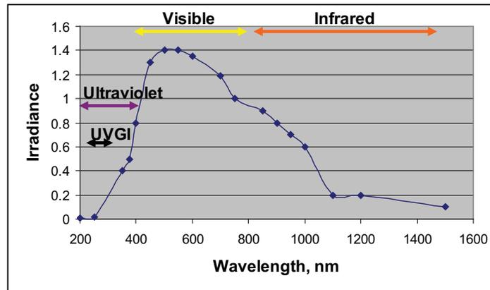
Figure 1-2. Solar spectrum showing UV and IR portion.
