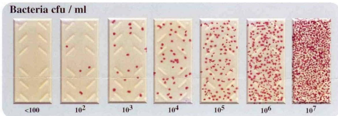
Figure 4-4. Pictorial scale for estimating bacteria level.
