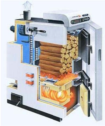
**Figure ES-3.** Under-burning solid wood boiler (Froeling 2005)
