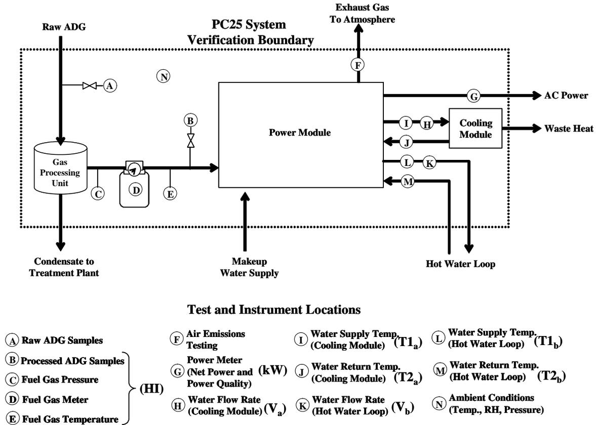
**Figure 1-3. Schematic of Measurement System**
