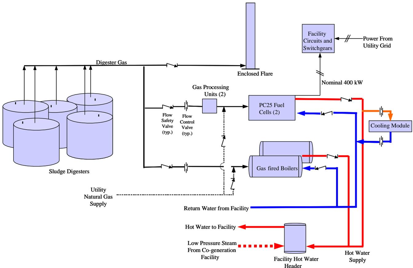
Figure 1-2. PC25C Integration Schematic for Red Hook WPCP
