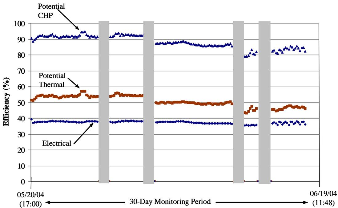
**Figure 2-3. PC25C Efficiency During the Extended Monitoring Period**
