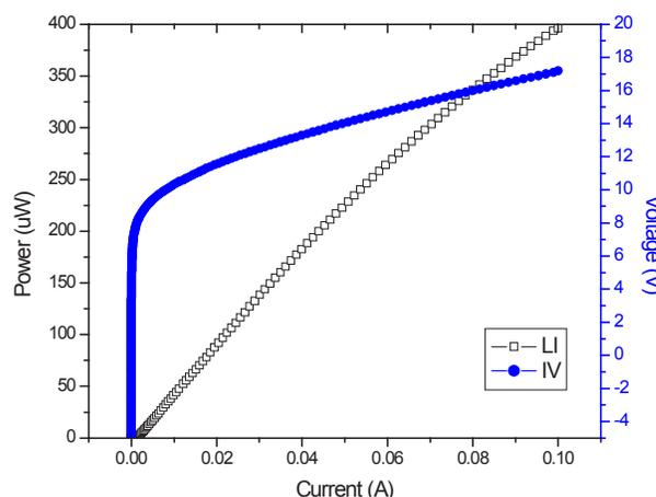
**Figure 3: Emission spectrum (left) and electrooptical characteristics (right) of a pseudomorphic ultraviolet LED.** The emission spectrum peaks at 265 nm, while the ultraviolet output power of the LED reaches 0.4 mW at 100 mA of injection current.
