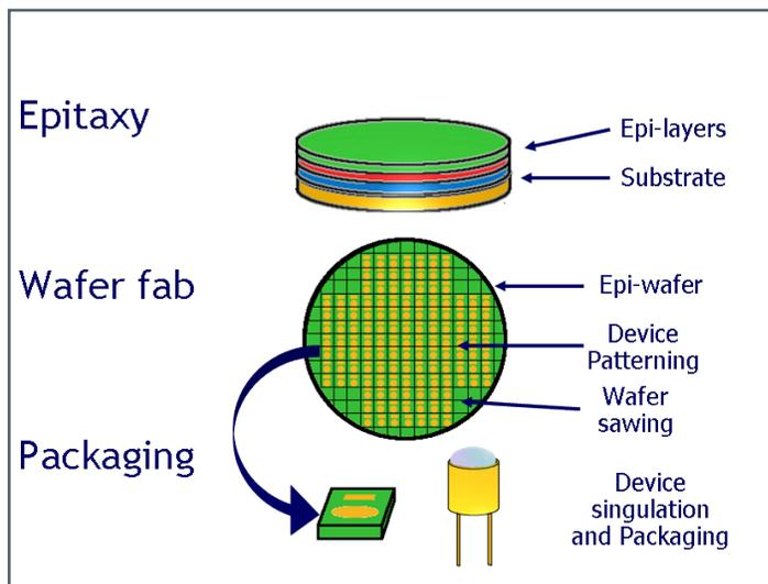
**Figure 1: Manufacturing a LED. Epitaxial deposition on the substrate; wafer fabrication (masking, etching, metallization, and device separation); device packaging (mounting, bonding of wires, and electrical connection of device to pins on package)**
