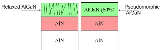
**Figure 2: Relaxed (left) and pseudomorphic (right) growth regimes for AlGaIn on AlN.** In the relaxed growth regime, the layer grows defect free up to a critical thickness after which strain is released through the formation of dislocations. In the pseudomorphic growth regime, although strained, the layer grows without generation of defects.
