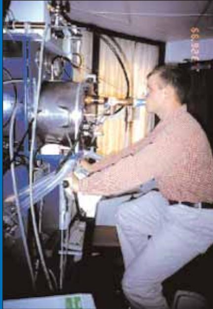
The ultrafine particle exposure system incorporated a bicycle to examine the effects of UFP exposure during exercise.
