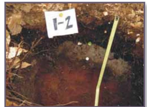
*Soil pits were excavated at each sampling location. Samples were collected of the O-horizon and upper B-horizon.*
