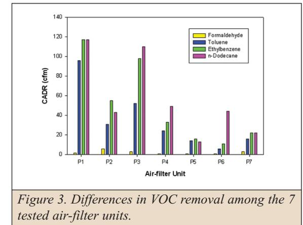
Figure 3. Differences in VOC removal among the 7 tested air-filter units.
