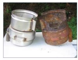
Corrosion due to combustion involving chlorine Photo Credit: BIOENERGY 2020+
