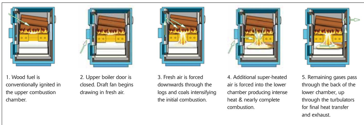
Figure 1. Example of staged combustion (courtesy of Econoburn).
