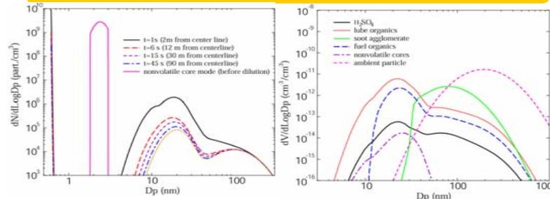
Fig. 4. (a) Number size distributions of NPs at four selected plume ages, and (b) volume size distributions for different components at plume age of 1 s for the case with the presence of refractory particles. The ambient T and RH are 295 K and 60%, respectively. ESC = 50 ppm and  $\epsilon = 2.5$  %.
