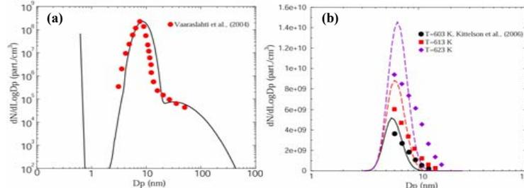
Fig. 1. Predicted particle size distributions and measured ones from (a) Vaaraslahti et al. (2004) and (b) Kittelson et al. (2006). The conversion efficiency  $\epsilon$  is assumed to be 53 %, 67 % and 72 % for exhaust temperature of 603 K, 613K and 623 K, respectively. The  $\epsilon$  used in Fig. 1 (a) is assumed to be 100 % for exhaust temperature of 750 K.
