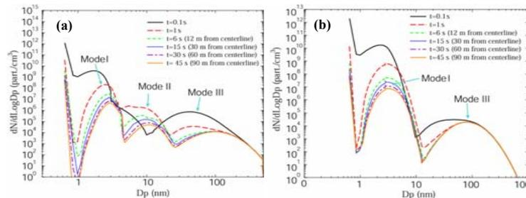
Fig. 2. NP formation and evolution as a function of plume ages up to 75 s under (a) high sulfur conditions (ESC=330 ppm with FSC=330 ppm) and (b) ultra-low sulfur conditions (ESC=30 ppm with FSC=15ppm and LSC=15ppm) in winter condition (T=278 K, RH=60 %). The lube oil sulfur content is assumed to be 3000 ppm and lube oil leaking rate is assumed to be 0.5 %. The conversion efficiency  $\epsilon$  is 1.4% for case (a) and 60% for case (b). Dilution is not corrected.
