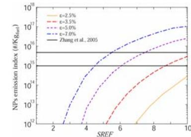
Fig. 3 NP emission indices as function of SREF at 4 different  $\epsilon$  (2.5 %, 3.5 %, 5.0% and 7.0 %) at ambient T=298 K and RH=50 %. The ESC is assumed to be 30 ppm.
