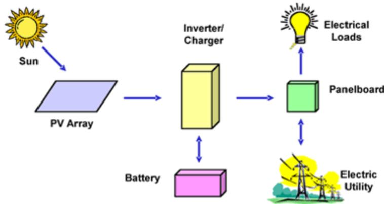
Figure 1. Solar photovoltaic (PV) system and typical components
