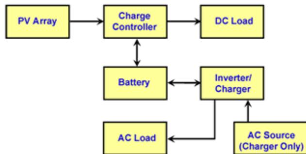
Figure 2. Stand-alone PV system with AC/DC loads.
