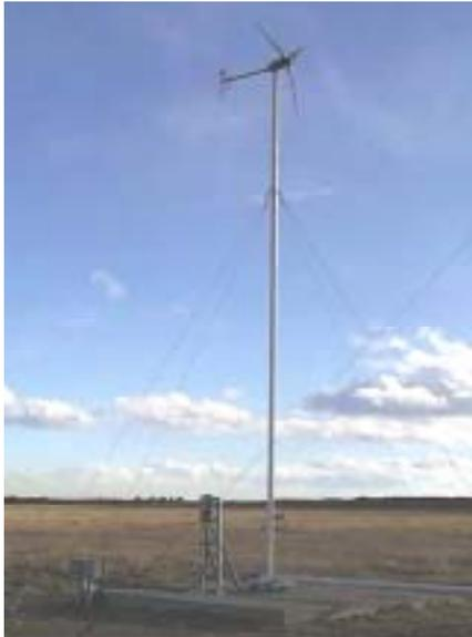
The *Whisper H40* (pictured above) is a three-blade upwind turbine with a rated power of 900 watts at a wind speed of 12.5 m/s. As tested, the turbine had its 24-volt DC output grid connected via a Trace SW4024 inverter. Power and over-speed control are by a patented “angle governor” that combines horizontal and vertical furling.
