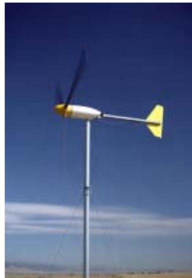
The Bergey *XL.1* (shown above) is a three-blade upwind turbine with a manufacturer's rated power of 1 kW at a wind speed of 11 m/s. A permanent magnet generator produces three-phase variable frequency output that is rectified to 24 volts DC. The turbine uses sideways furling for over-speed protection. It has a rotor diameter of 2.5 m and a hub height of 9 m. The microphone at the reference position was located at a slant distance of 13.8 m.
