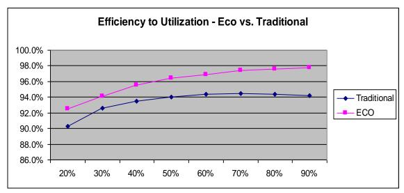
Figure 9 - UPS Utilization to Efficiency
