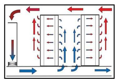
Figure 5 - Cold Aisle Containment
