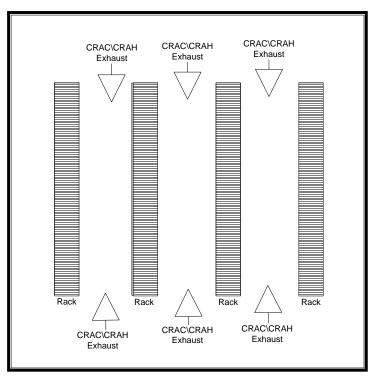
Figure 8 - CRAC\CRAH Placement
