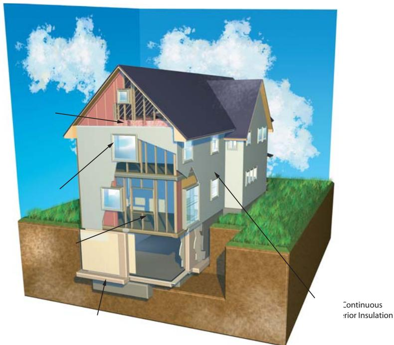
Ideally, the Solar Heat Gain Coefficient (SHGC) should be specified for windows of different orientations. The SHGC is a measure of how well a window absorbs or reflects heat from the sun. The lower the coefficient, the better the window is at blocking the sun's heat. Windows should be specified with low (<.4) SHGC on west-facing orientations in particular to reduce summer over-heating, and higher SHGC should be specified on south-facing windows.
