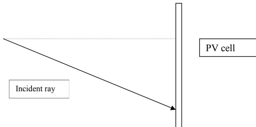
The horizontal line equals the length of the incident ray times the sine of the angle between the incident ray and the photovoltaic cell. It is the component of the incident ray that is perpendicular to the photovoltaic cell.
