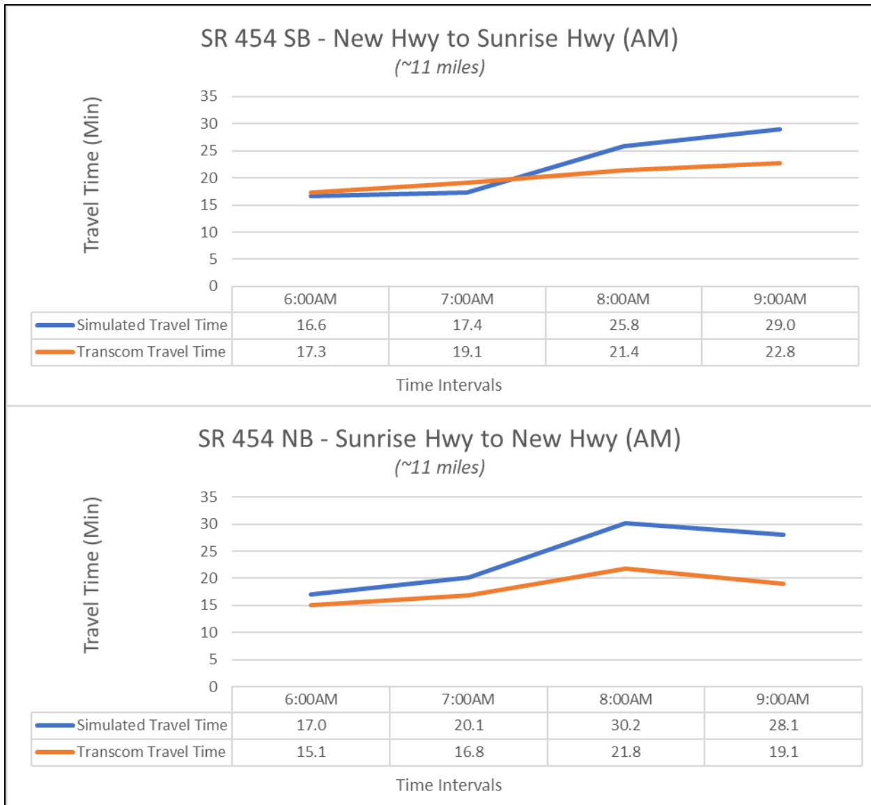
Figure A-12. AM Travel Time Validation—SR 454 from New Hwy to Sunrise Hwy
